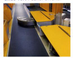
This cam bladed device transfers baggage from one line to another, or to a sorting destination, at a rate of 60 bags per minute, whilst maintaining the gentlest treatment of baggage through the unique constant velocity curved shape.
