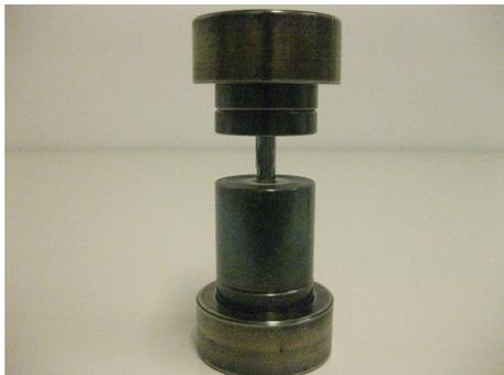
**Figure 5.2:** Mounted sample press.
