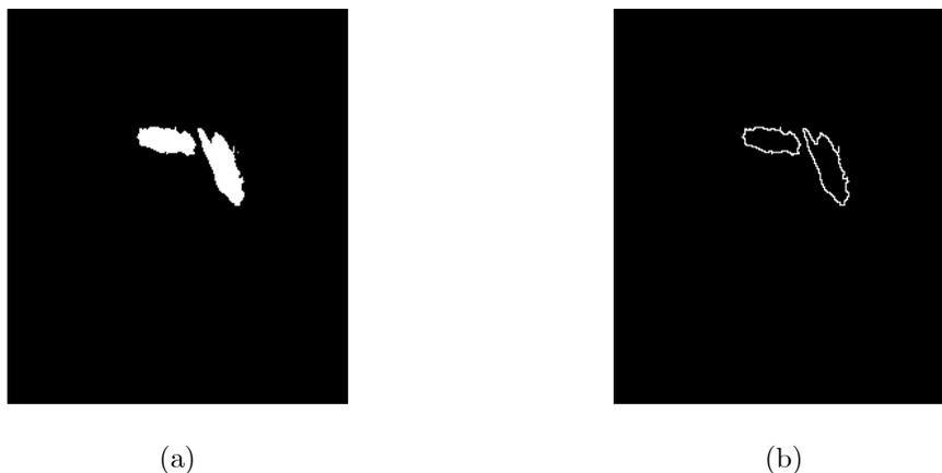
Figure 33: (a) bwImage of the two regions before Occlusion. (b) extracted characteristic information  $\mathfrak{C}$  for method *boc*
