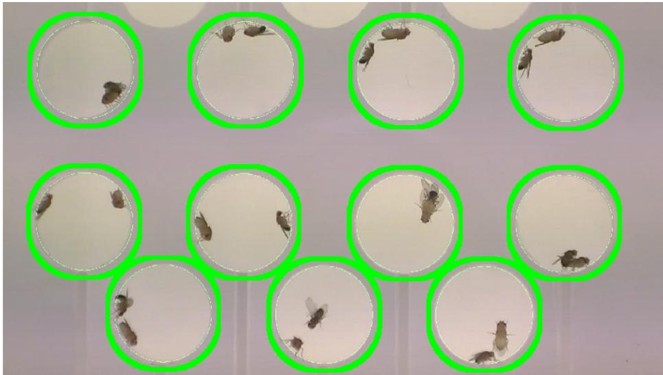
Figure 16: Snapshot of a video with detected arenas and watched boundary rings (in green).
