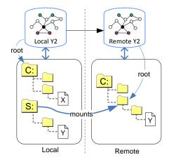
Figure 9.4: Mounting remote Y2 metadata storages.
