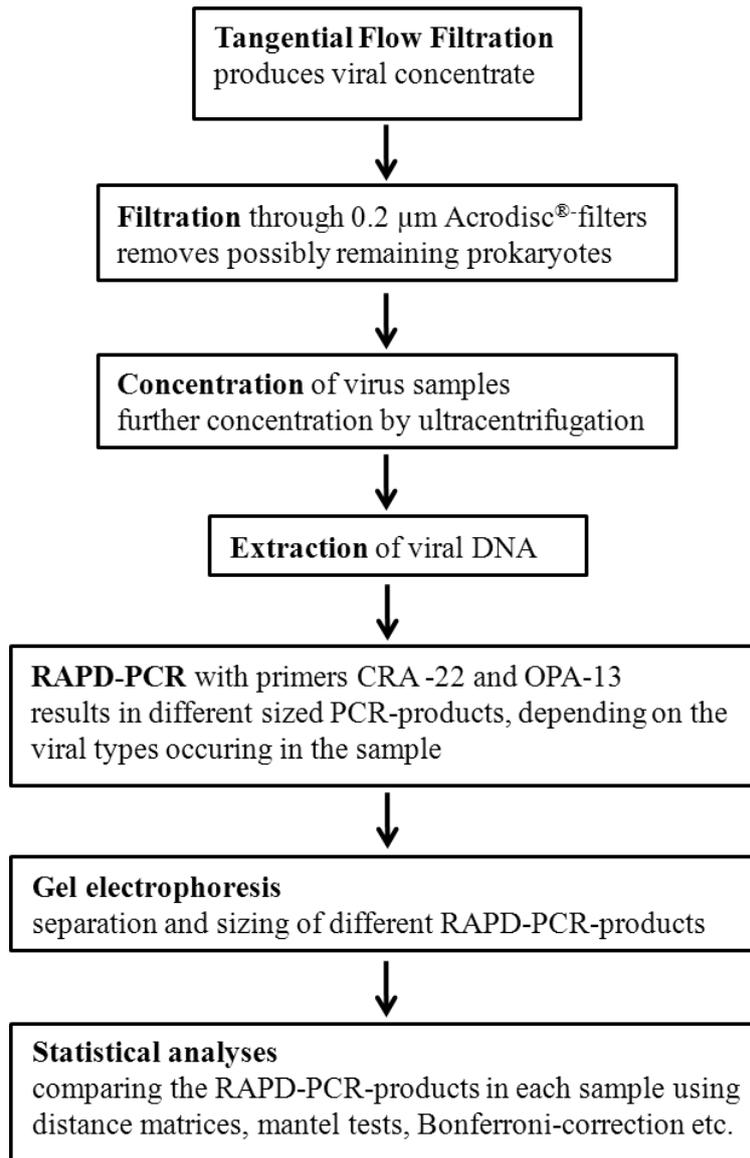
Figure 7 Schematic overview of the specific steps of RAPD-PCR. Tangential Flow Filtration was performed on the ship, filtration through 0.2 µm-filters and subsequent steps were performed in Vienna.
