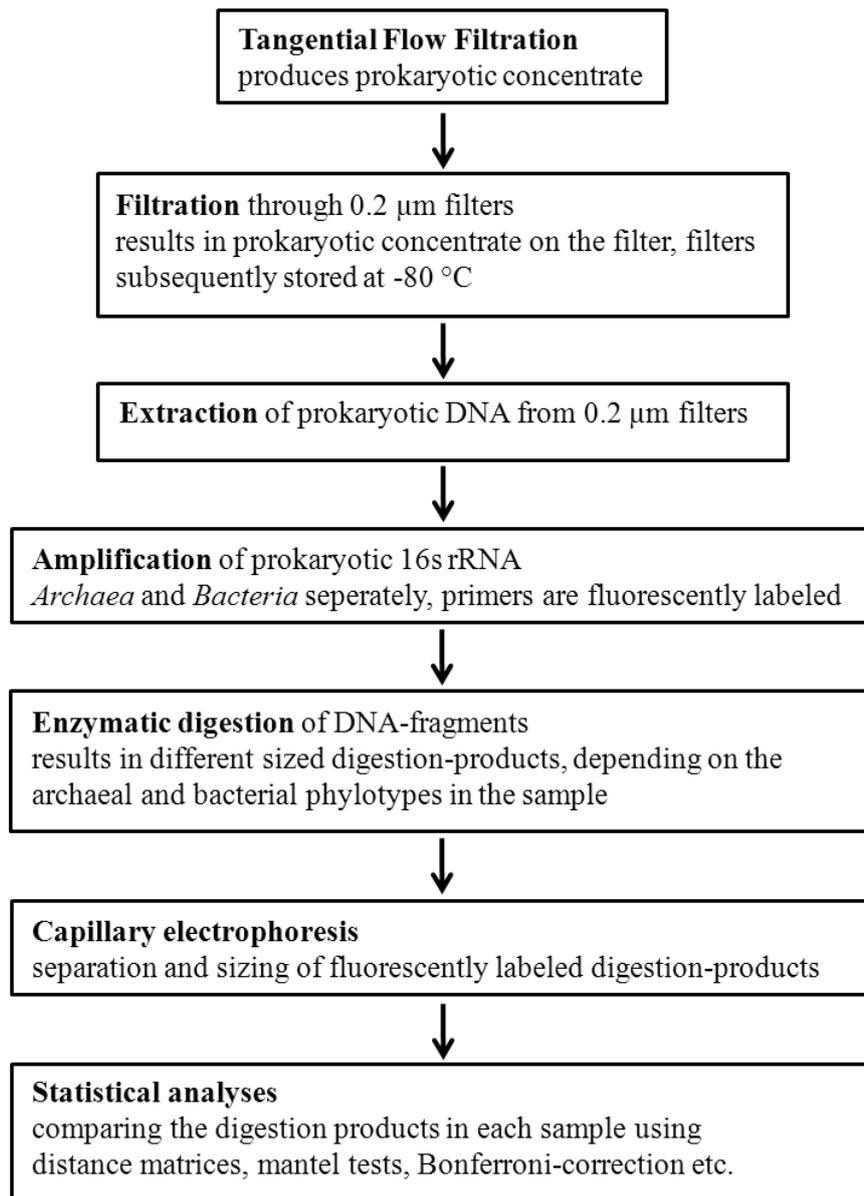
Figure 6 Schematic overview of the specific steps of T-RFLP. Tangential Flow Filtration and filtration through 0.2 µm-filters were performed on the ship, subsequent steps were performed in Vienna.
