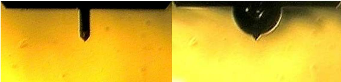
*Fig. 3.48: (left) Top view of silicon cantilever in water several micrometers away from a thin film gold surface. (right) Bubble formation due to water oxidation in the high electric field at the end of the SPM tip.*
