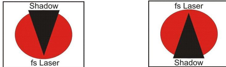
*Fig. 3.29: Image of the tip shadow on the screen due to the different focal position relative to the tip. On the left picture the focal point is in front of the tip whereas on the right side it is behind the tip.*
