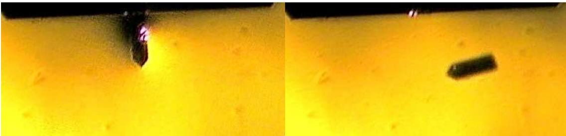
*Fig. 3.49: (left) Top view of the cantilever directly before it is blown up by the shock wave produced by the water breakdown. The scattered light already indicates changes in the laser beam path. (right) Floating cantilever after detachment from the holder.*
