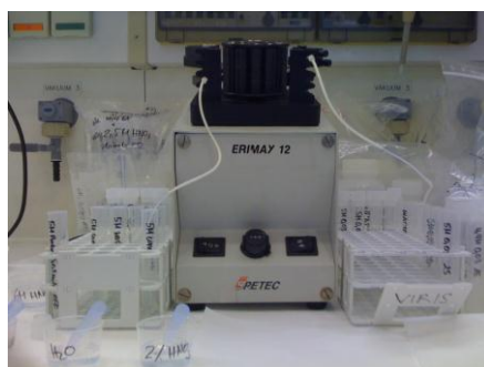
Fig. 12 Peristaltic Pump Experimental Setup
