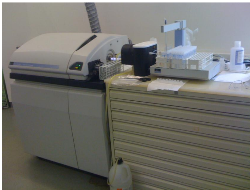
Fig. 7 Measurement Setup ELAN DRc with APEX and autosampler
