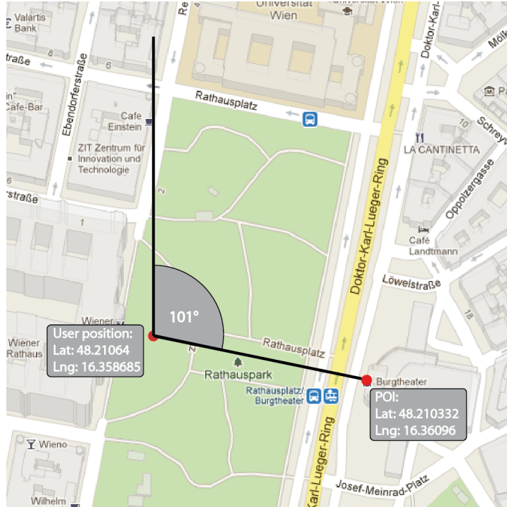
FIGURE 4.6: Bearing between two points
