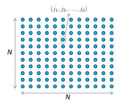
**Figure 3.2:** A *d*-dimensional cubic lattice with *N* sites per side. Each site is identified by a set of integers  $\vec{j} = (j_1, j_2, ..., j_d)$ , each running between 1 and *N*, and corresponds to the equilibrium position of a quantum harmonic oscillator with Hilbert space  $\mathcal{H}_{\vec{j}}$ . The full system has thus Hilbert space  $\mathcal{H} = \bigotimes_{\vec{i}} \mathcal{H}_{\vec{j}}$ . In the picture, d = 2.
