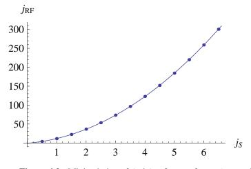
**Figure 4.2:** Minimal size of (spin) reference frame  $j_{RF}$  needed for violation of the Bell inequality for measurements on a pair of entangled spins of size  $j_S$ . The dots are calculated numerically, the line is the extrapolated fit  $j_{RF} \simeq 6j_S^2 + 6j_S$ .
