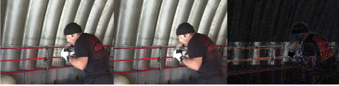
Figure 7: Patched slice for error concealment. From left to right: reference frame, patched frame, difference between frames.
