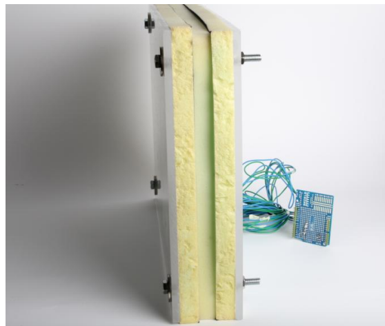
Figure 2. The wired prototype. The rightmost part can be mounted on a chimpanzee enclosure. The animals come in contact with the leftmost side.
