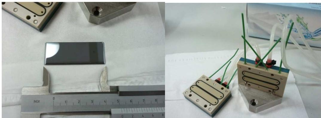
**Fig. 5. (left) Silicon ATR multiple internal reflection element (MIRE). (right) Teflon MIRE holder with fluid chambers, tubings and o-rings.**
