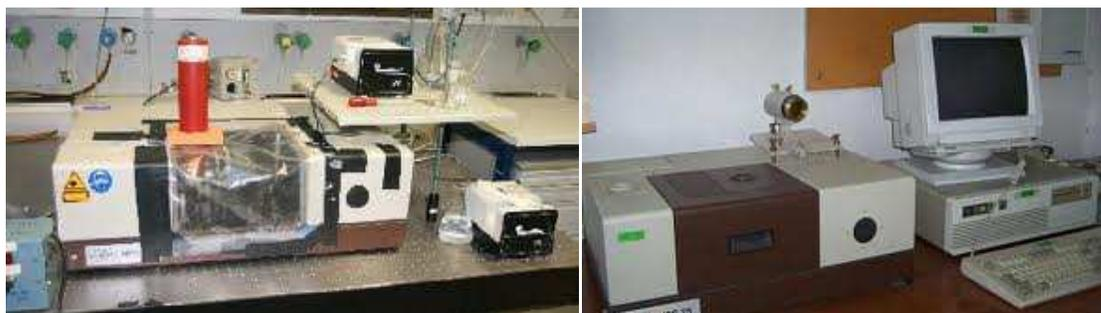
**Fig. 6. (left) IFS 66 spectrometer with detector (red) and attached peristaltic pumps. (right) IFS 25 spectrometer. (bottom) schematics of an FTIR-ATR spectrometer.**
