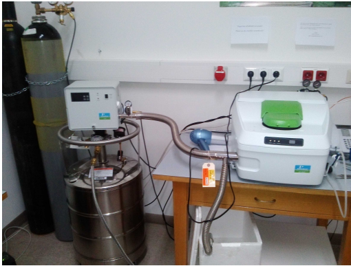
(a) Instrumental setup of the Perkin Elmer DSC 8500 with liquid nitrogen tank for the cooling and nitrogen as purge gas.
