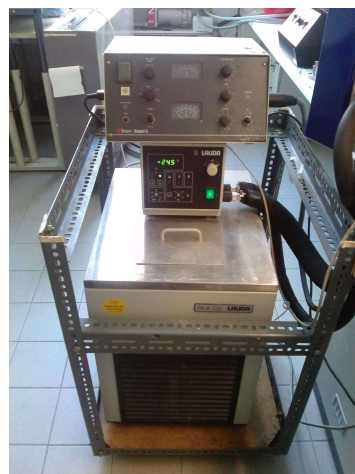
(c) Lauda RK 8 CS cooling regulator for the electrolyte.
