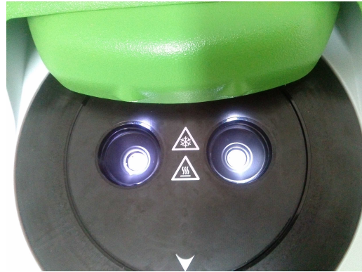
(b) Crucibles inside the furnaces of the Perkin Elmer DSC 8500, the left is the specimen chamber, the right one the reference chamber.
