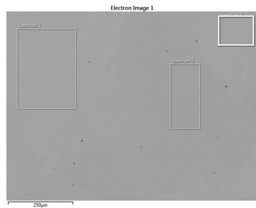
(b) Secondary electron detector SEM image of \text{Co}_3\text{Ti} - The regions show the areas from which the spectra are recorded.
