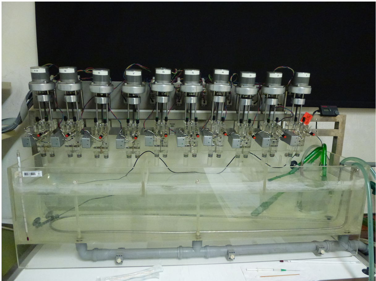
Abb. 7: Automatisch registrierendes Mikrorespirometer (Eigenbau IFFF).
