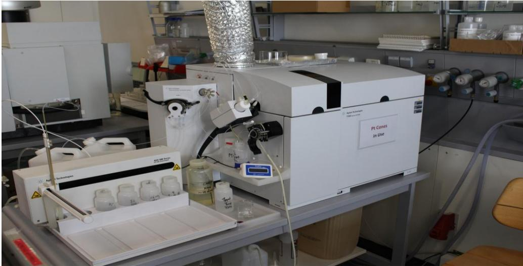
Abb. 19: Verwendete ICP-MS
