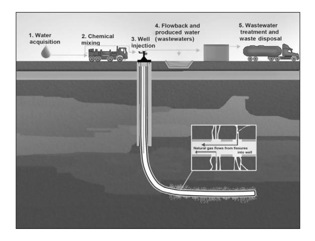
Image 3-1: EPA, Bahadori, "hydraulic fracturing water cycle" (2014)
