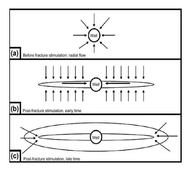
Image 1-4: Wang, J. et.al., "Gas flow mechanism before and after fracking" (2012)
