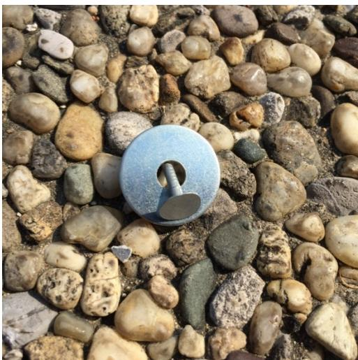
**A.15.** artificial substratum (nail and washer) for calcium carbonate precipitation rate.
