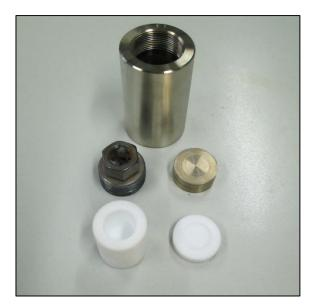
Figure 2. Morey-autoclave with Teflon vessel.
