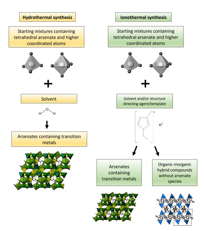
Figure 8. A schematic illustration of the synthesis of tetrahedral-octahedral frameworks under hydrothermal (left) and ionothermal (right) conditions.
