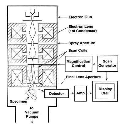
Figure 6. A schematic diagram of an electron column (Goldstein et al., 2003).
