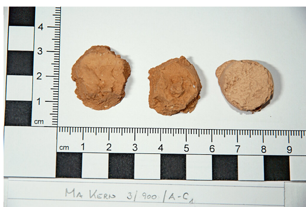
(a) Samples fired for 3 hours at peak temperature 900°C
