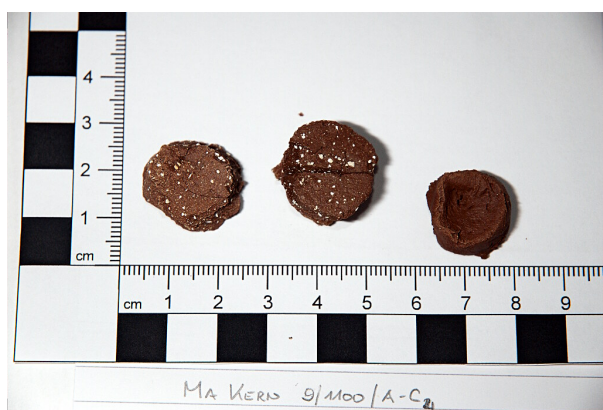
(c) Samples fired for 7 hours at peak temperature 1100°C
