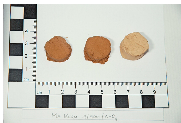
(d) Samples fired for 9 hours at peak temperature 900°C
