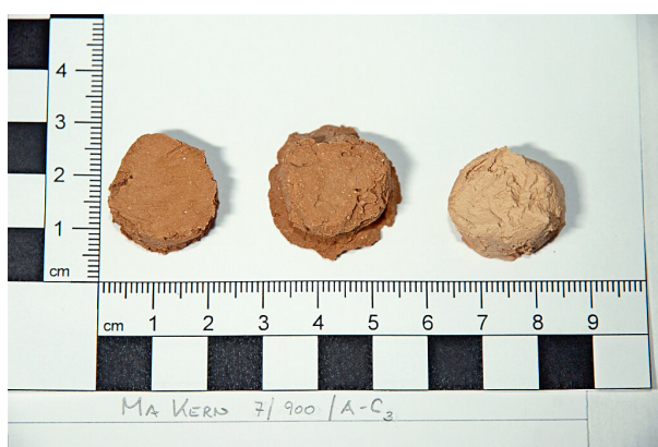
(c) Samples fired for 7 hours at peak temperature 900°C
