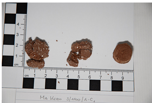
(a) Samples fired for 3 hours at peak temperature 1100°C
