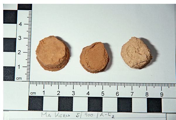
(b) Samples fired for 5 hours at peak temperature 900°C
