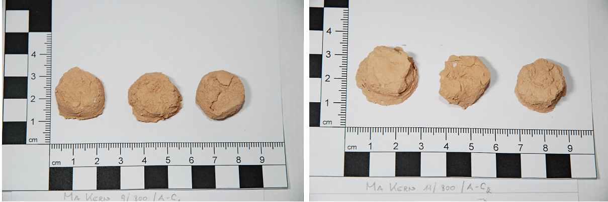
(a) Samples fired for 9 hours at peak temperature 800° C (b) Samples fired for 11 hours at peak temperature 800° C
