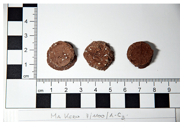
(d) Samples fired for 9 hours at peak temperature 1100°C
