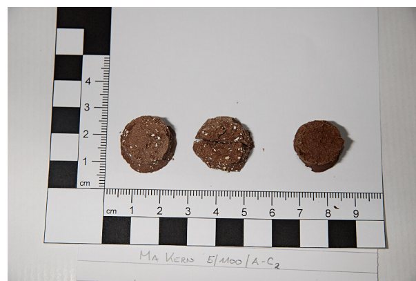
(b) Samples fired for 5 hours at peak temperature 1100°C
