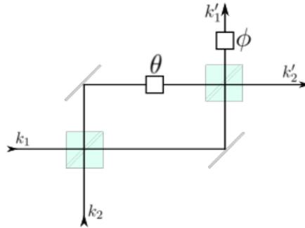
Figure 3.1: A Mach-Zehnder interferometer can be used to implement any non-standard beam splitter, by the modulation of two phase shifters  $e^{\theta i}$  and  $e^{\phi i}$  (labelled with  $\theta$  and  $\phi$ , respectively).
