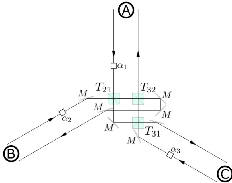
Figure 3.2: A possible experimental arrangement of the three-party game. The operator TS has been decomposed into elementary optical devices, i.e. beam splitters ( $T_{32}$ ,  $T_{31}$  and  $T_{21}$ ) and phase shifters ( $\alpha_1$ ,  $\alpha_2$  and  $\alpha_3$ ). The apparatus is supplemented by mirrors ( $M$ s) that serve to guide the photons from A, B, C towards the center (where TS is implemented) and back to players.
