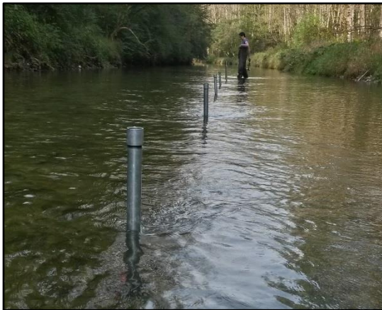
Figure 8. Left: set up of open-bottom K_v -measurements at the central axis of a stream segment; right: stock picture of the CMD-2 conductivity meter, http://www.gfinstruments.cz , CZ.
