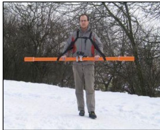
Figure 8. Left: set up of open-bottom K_v -measurements at the central axis of a stream segment; right: stock picture of the CMD-2 conductivity meter, http://www.gfinstruments.cz , CZ.
