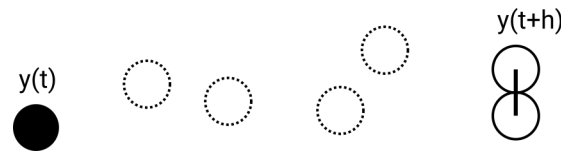
Figure 11: Starting from y(t) , the RKCK method constructs help-points (dotted circles) to derive the 4th and 5th order solutions for y(t + h) . If the error (indicated by the line) is smaller than a given tolerance, the step is accepted.
