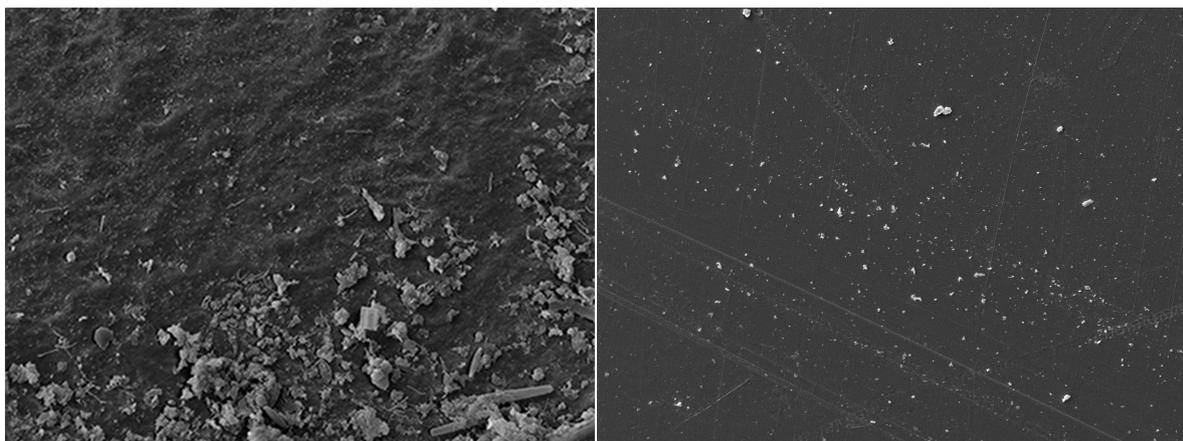
**Supplementary Figure 3** - Scanning electron microscopy pictures. Left: PVC DEHP light, after one week of incubation; Right: PP dark, after one week of incubation. Both pictures were taken at 450x magnitude. The PVC picture (left) shows clear waves in the upper left corner, while the surface of the PP (right) is completely smooth
