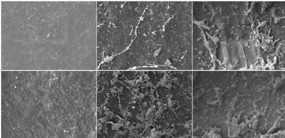
**Figure 8** - SEM pictures showing HDPE samples throughout the entire incubation time. The upper panels show the light and the lower panels the dark conditions. Columns from left to right: HDPE after one week, HDPE after one month, HDPE after two months of incubation.
