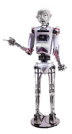
RoboThespian can either act on its own with the help of preprogrammed scripts or via teleoperation. When in autonomous use, the robot uses all features it has been programmed with including its communication capabilities. It can blink, squint with its eyes and use prerecorded audio files. In the case of teleoperation, the operator can "command the robot to use simple movements, such as turning, basic gesture, and live interaction" (Verner et al. 2016. 76). Furthermore, the operator can choose
