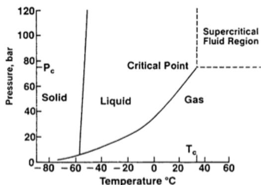
**Figure 6:** Phase diagram for carbon dioxide
