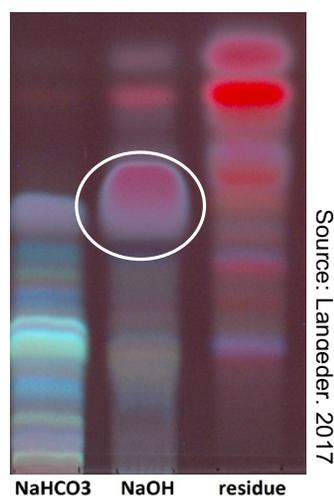
**Figure 3:** TLC-fingerprint comparison of  $\text{NaHCO}_3$ -fraction, Residue-fraction and  $\text{NaOH}$ -fractions (high accumulation of diterpenes is marked)
