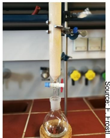
Figure 5: Dowex Marathon WBA, during the exchange of ions
