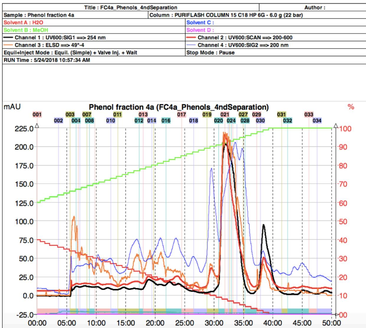
Figure A 9: Flash chromatogram FC04b of the Phenol fractions
