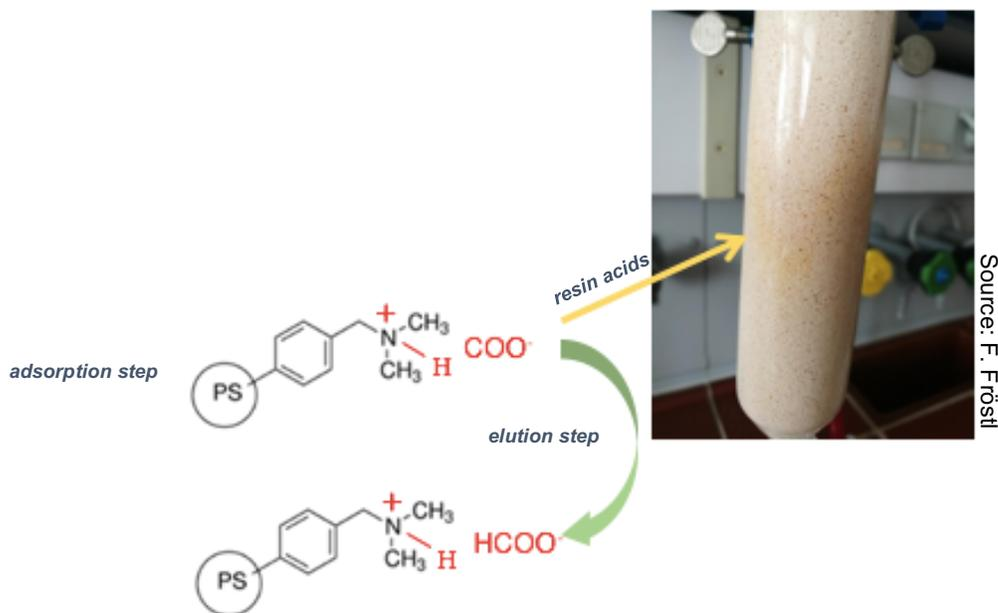
**Figure 7:** The attached acids in the column (right) and the process of displacement of the resin acid (COO<sup>-</sup>) by the formic acid (HCOOH) during the elution step (left)
