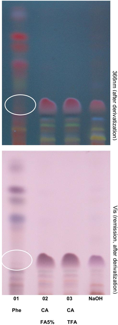
**Figure 12:** TLC comparison, showing the depletion of resin acids in the phenol fraction (encircled area)
