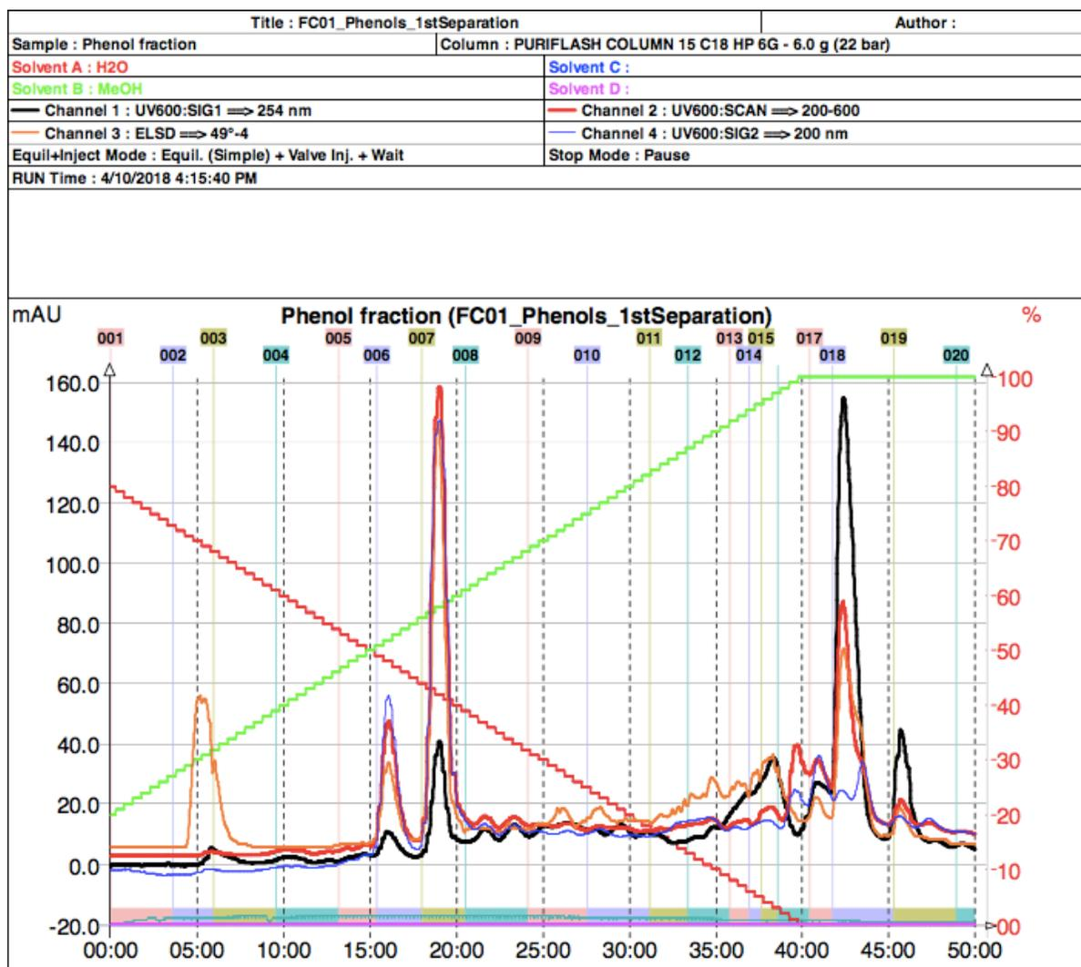
Figure A 6: Flash chromatogram 02 of the Phenol fractions
