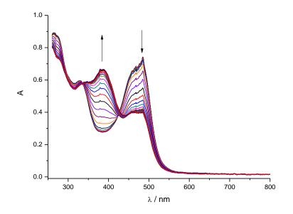
Figure 25: Evolution of UV–vis spectra in 2D projection in forward scan observed for  $[Cu_3Cl_2(\mu-Cl)_2(HL^1)_3]Cl_2$  in DMSO/nBu<sub>4</sub>NPF<sub>6</sub> in the region of the first cathodic peak (scan rate of 10 mV s<sup>-1</sup>, Pt-microstructured honeycomb working electrode).
