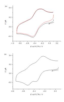
Figure 27: Cyclic voltammograms of iron complexes (a)  $[Fe(HL^2)_2]Cl_3$  and (b)  $[Fe(HL^1)_2]Cl_3$  in DMSO/nBu<sub>4</sub>NPF<sub>6</sub> at scan rate of 100 mV s<sup>-1</sup> and at GC working electrode (black traces represent the first scan, while red trace the second scan).
