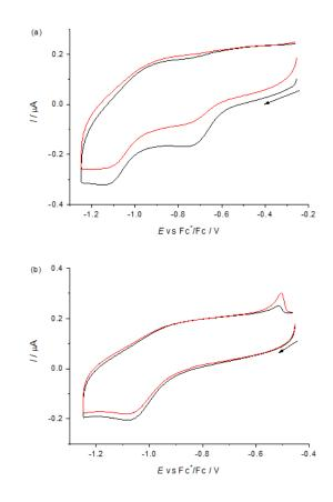
Figure 24: Cyclic voltammograms of (a)  $[Cu_3Cl_2(\mu-Cl)_2(HL^1)_3]Cl_2$  and (b)  $[Cu(L^2)Cl]^0$  in DMSO/nBu<sub>4</sub>NPF<sub>6</sub> at scan rate of 100 mV  $s^{-1}$  and at GC working electrode (black traces represent the first scan, while red traces the second scan).
