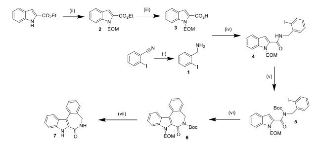
Scheme 1: Synthesis pathway to achieve the underivatised indolobenzazepine; (i): Argon, THF, 0°C, 80°C; (ii): Argon, DMF, 0°C, RT; (iii): Ethanol, LiOH·H₂O, reflux; (iv): Argon, DCM, 0 °C, RT; (v): Argon, MeCN, RT; (vi): Argon, DMF, 100 °C; (vii): Dioxane, 1N HCl, reflux
