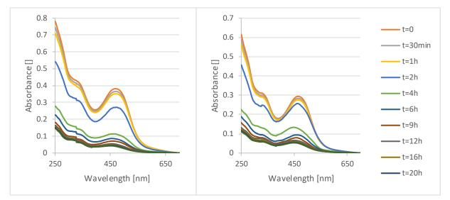
Figure 23: UV-vis measurements over time from 0 to 20 hours; left: [Cu<sub>3</sub>Cl<sub>2</sub>(µ-Cl)<sub>2</sub>(HL<sup>1</sup>)<sub>3</sub>]Cl<sub>2</sub>, right: [Cu<sub>1</sub>L<sup>2</sup>)Cl<sub>2</sub><sup>0</sup> in 154 mM NaCl
