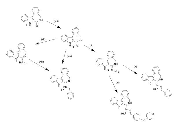
Scheme 2: Synthesis pathway of the three desired ligands; (viii): Argon, MeCN, Al<sub>2</sub>O<sub>3</sub>·P<sub>4</sub>S<sub>10</sub>, reflux; (ix): H<sub>2</sub>N-NH<sub>2</sub>·H<sub>2</sub>O, 135°C, (x): Argon, Ethanol, Picolinaldehyde, 95°C; (xi): Argon, Ethanol, 5-(morpholinomethyl)picolinaldehyde; 90°C; (xii): Argon, NaH, THF, MeI, reflux; (xiii) and (xiv) showed no conversions
