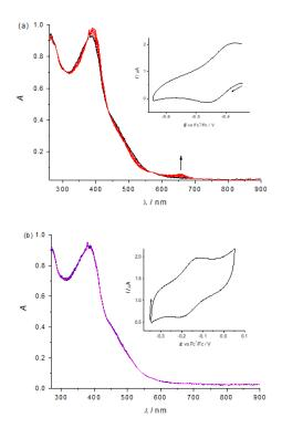
Figure 29: UV-vis spectra detected simultaneously during spectroelectrochemistry of [Fe(HL<sup>1</sup>)<sub>2</sub>]Cl<sub>3</sub> in nBu<sub>4</sub>NPF<sub>6</sub>/DMSO (a) in the region of the first cathodic peak and (b) in the region of the first anodic peak (insets: corresponding cyclic voltammograms, Pt-microstructured honeycomb working electrode, scan rate v = 5 mV s<sup>-1</sup>).
