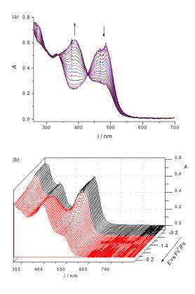
Figure 26: In situ UV-vis-NIR spectroelectrochemistry for **[Cu(L<sup>2</sup>)Cl]**<sup>0</sup> in DMSO/nBu<sub>4</sub>NPF<sub>6</sub> (scan rate of 10 mV s<sup>-1</sup>, Ptmicrostructured honeycomb working electrode): (a) evolution of UV-vis spectra in 2D projection in forward scan; (b) UV-vis spectra detected simultaneously upon the cyclic voltammetric scan in 3D projection.
