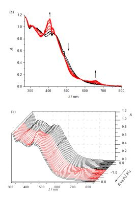
Figure 28: Spectroelectrochemistry of  $[Fe(HL^2)_2]Cl_3$  in nBu<sub>4</sub>NPF<sub>6</sub>/DMSO in the region of the first cathodic peak. (a) UV-vis spectra detected simultaneously during the in-situ reduction (Pt-microstructured honeycomb working electrode, scan rate v = 10 mV s<sup>-1</sup>); (b) potential dependence of UV-vis spectra.
