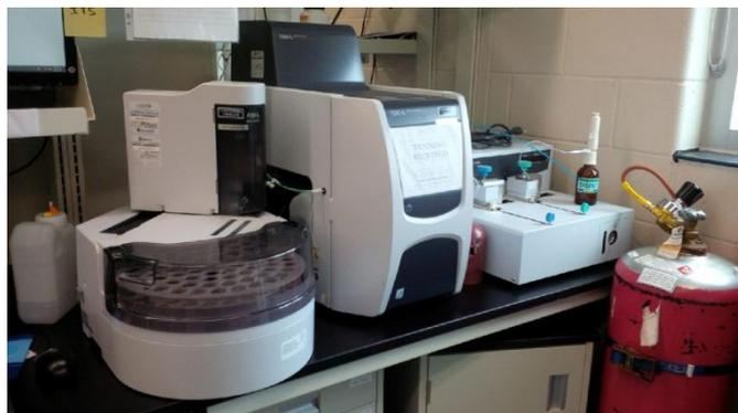
Abbildung 37 TOC-Analyser (Quelle: <https://navigator.innovation.ca/en/facility/wilfrid-laurier-university/center-cold-regions-and-water-science>)
