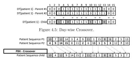
Figure 4.6: Position-based Crossover Operator.
