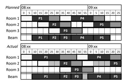
Figure 5.4: Exemplary Planned Schedule and Actually Executed Schedule (white: preparation times; dark gray: irradiation times; medium gray: exiting times); light gray: pre-beam waiting times.
