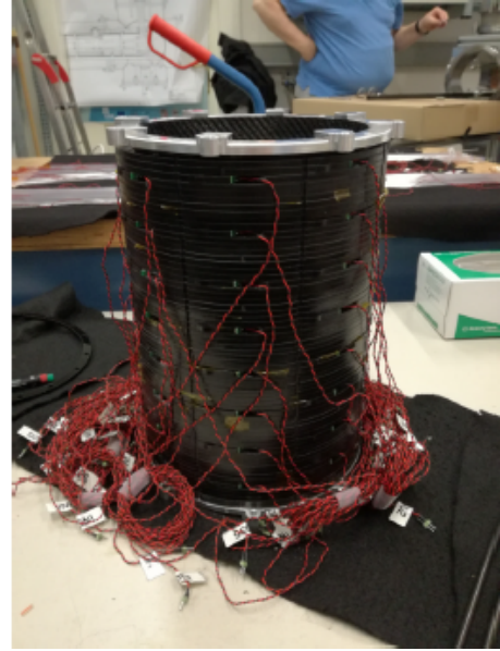
(b) The inner layer of the fiber upgrade, fully assembled.
