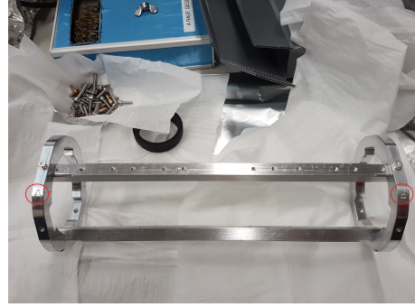
(b) Attaching end-piece “E”. Note how the markings “A” and “E” are aligned.
