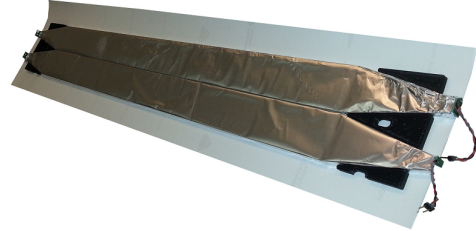
(b) A view of an outer hodoscope segment. The scintillating bars are wrapped in aluminum foil separately before being grouped up and wrapped in light blocking foil.
