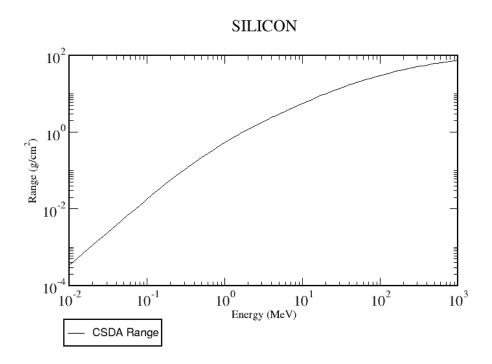
FIGURE 7: CDSA Range as function of the energy for electrons in silicon (reprinted from *NIST database*, retrieved from https://www.nist.gov/pml/stopping-power-range-tables-electrons-protons-and-helium-ions (9.2.19))
