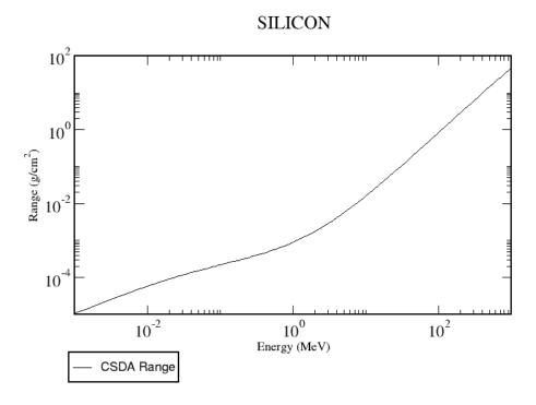
FIGURE 8: CDSA Range as function of the energy for helium ions in silicon (reprinted from *NIST database*, retrieved from https://www.nist.gov/pml/stopping-power-range-tables-electrons-protons-and-helium-ions (9.2.19))
