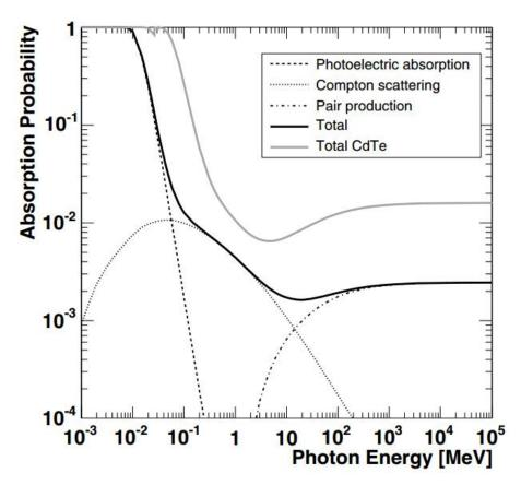
FIGURE 9: Total absorption probability of photons from  $\gamma$ -transformatios and X-ray radiation in a 300 $\mu$ m thick silicon (solid black) and CdTe (solid grey) for comparison (retrieved from [21] as reprinted from Rossi, L. et al. (2006). Pixel Detectors. Berlin: Springer)
