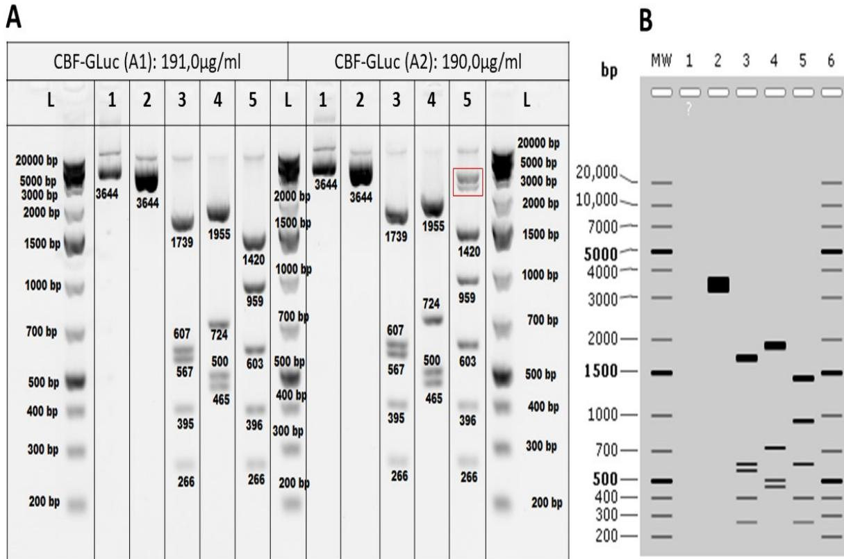
Figure 24: Agarose gel electrophoresis of CBF-GLuc (A) and the simulation on Snap Gene® (B).
