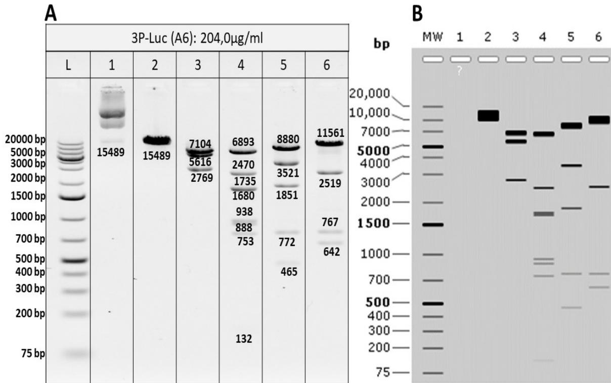
Figure 31: Agarose gel electrophoresis of 3P-Luc (A) and the simulation on Snap Gene® (B).
