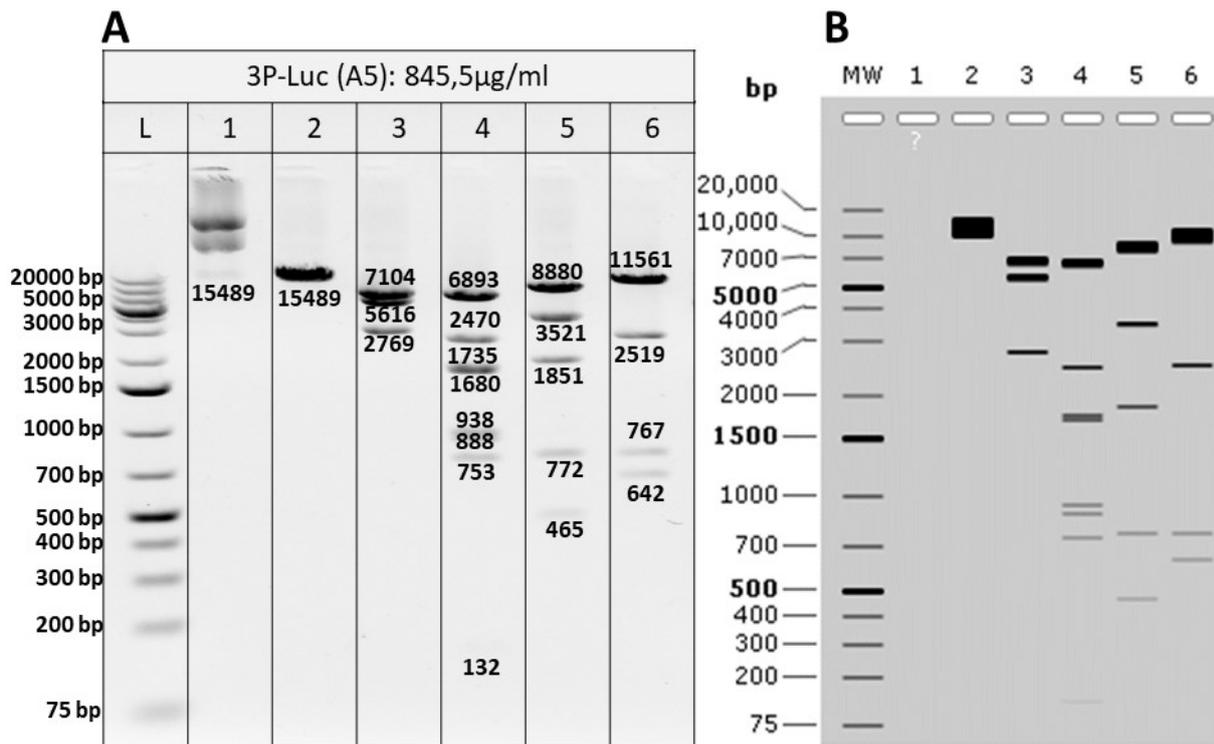
Figure 30: Agarose gel electrophoresis of 3P-Luc (A) and the simulation on Snap Gene® (B).
