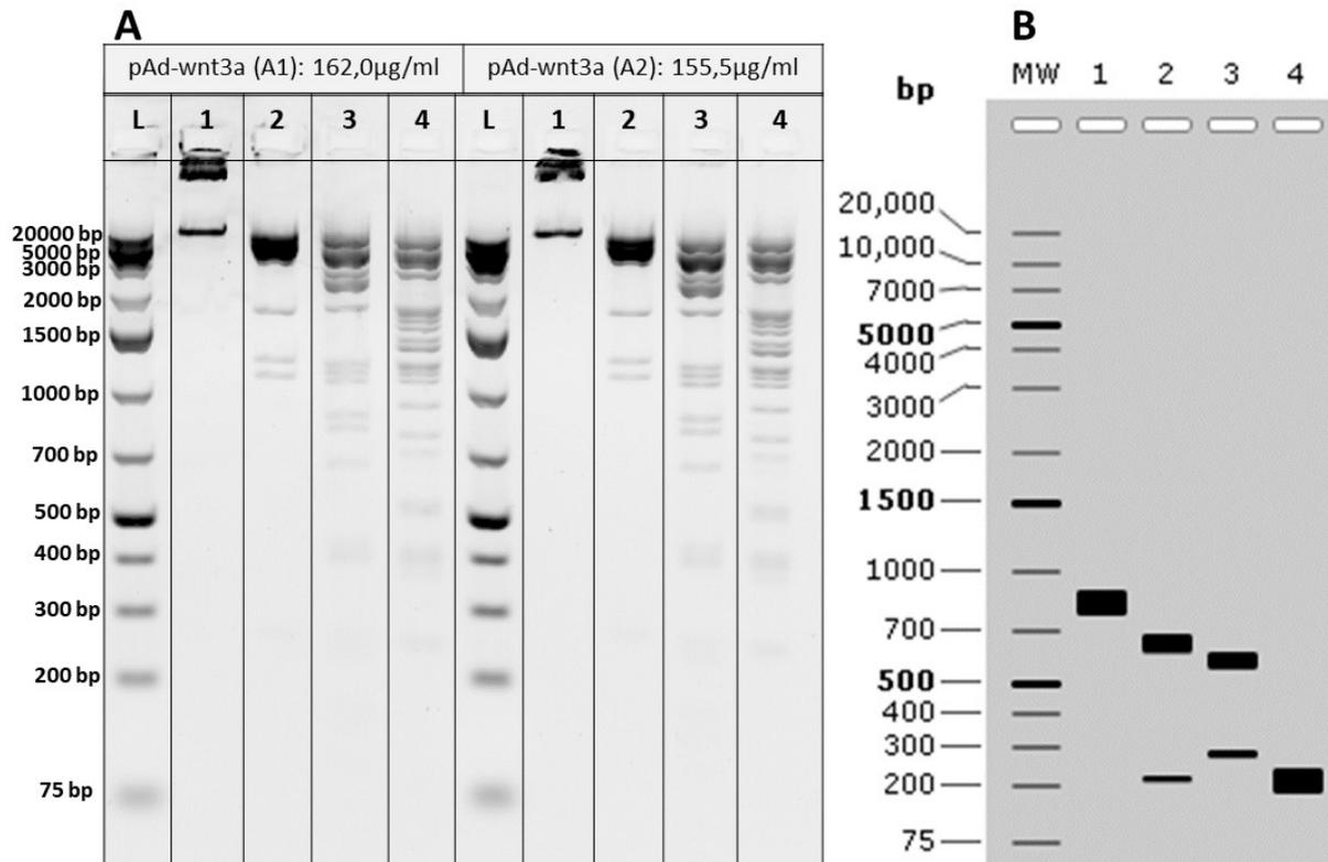
Figure 41: Agarose gel electrophoresis of pAd-wnt3a (A) and the simulation on Snap Gene® (B).
