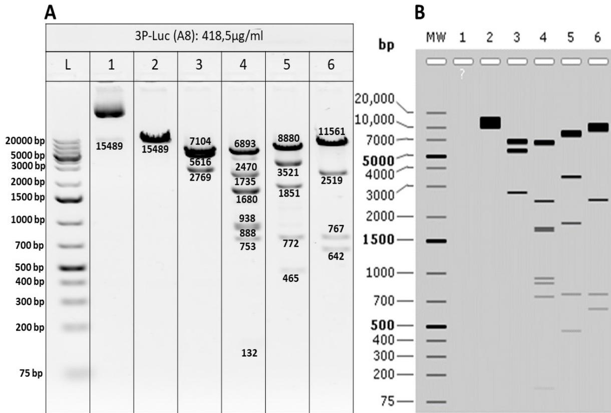
Figure 33: Agarose gel electrophoresis of 3P-Luc (A) and the simulation on Snap Gene® (B).
