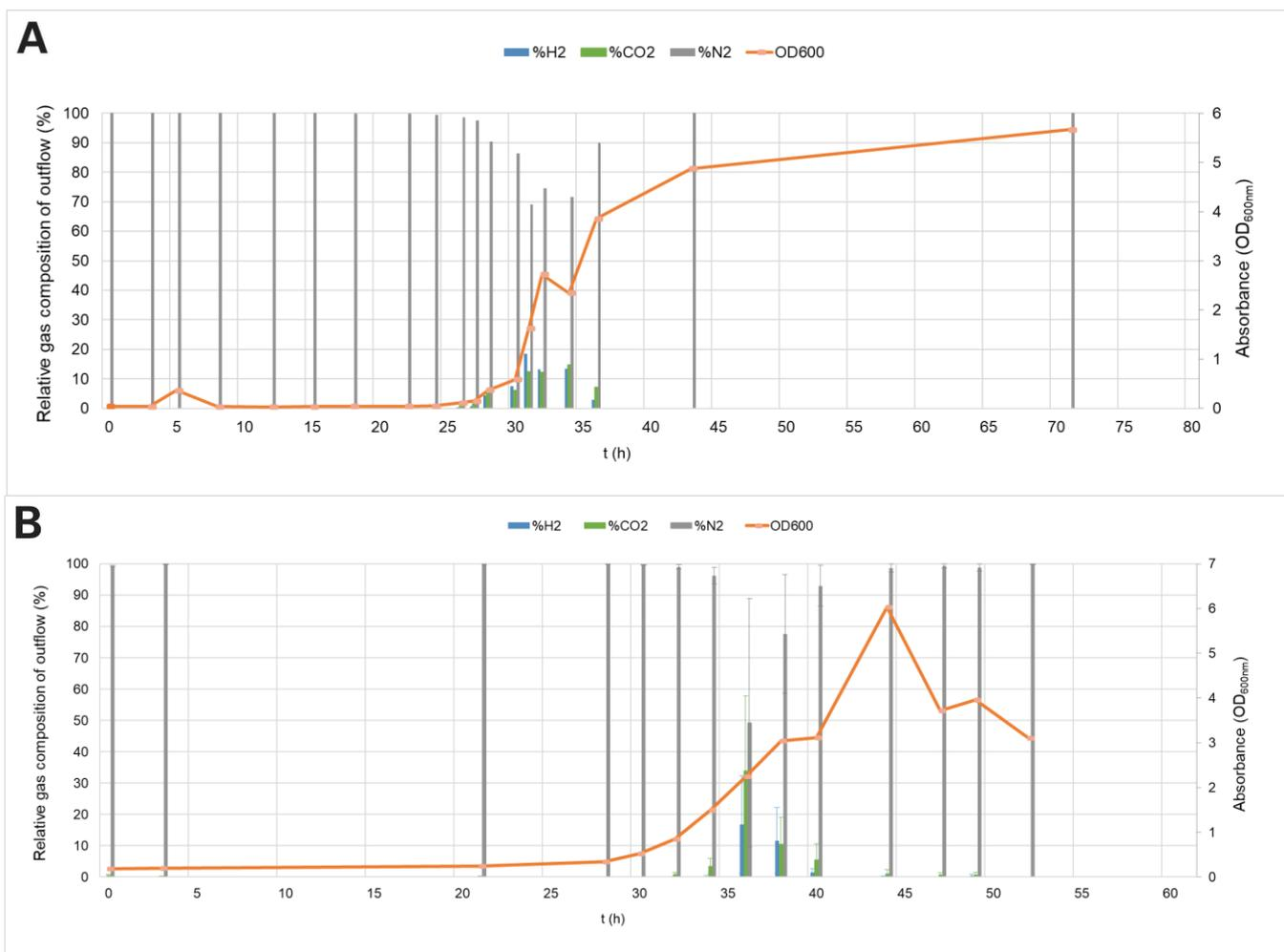
**Fig. 15** GC results over time with relative ratio of H<sub>2</sub> (blue bars), CO<sub>2</sub> (green bars) and N<sub>2</sub> (grey bars) in combination with OD<sub>600</sub> (orange) of *C. acetobutylicum* (Clostridium medium) (**A**) and *E. aerogenes* (Delisa medium) (**B**) under pH-controlled conditions. Standard deviations are shown for the mean values.
