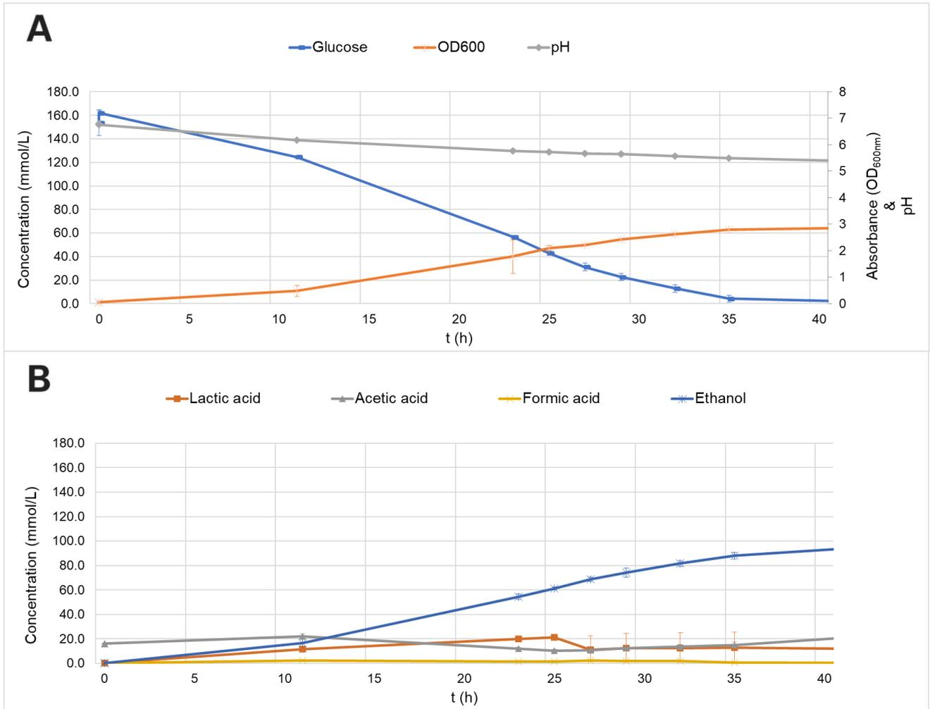
**Fig.14** HPLC results of liquid metabolites in batch samples of co-cultured *C. acetobutylicum* and *E. aerogenes* in DOE E medium under pH-uncontrolled conditions, showing concentrations (mmol/L) over time (h). **A** shows the glucose concentration combined with OD<sub>600</sub> and pH-level of medium over time. **B** shows VFA concentrations of lactic acid, acetic acid, formic acid and ethanol over time. Standard deviations are shown for the mean values.
