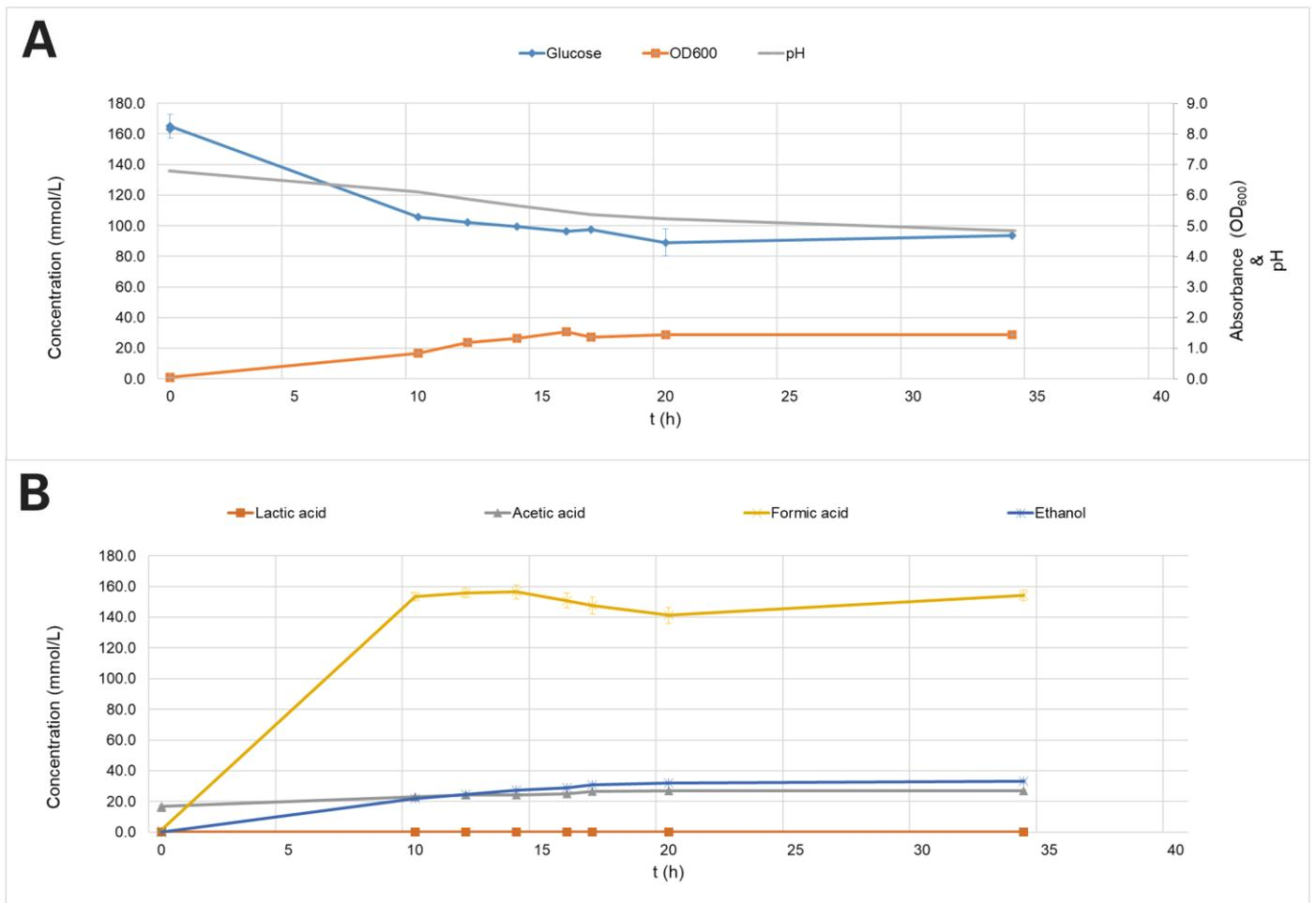
**Fig.11** HPLC results of liquid metabolites in batch samples of *E. aerogenes* in DOE E medium under pH-uncontrolled conditions, showing concentrations over time. **A** shows the glucose concentration combined with OD<sub>600</sub> and pH-level of medium over time. **B** shows VFA concentrations of lactic acid, acetic acid, formic acid and ethanol over time. Standard deviations are shown for the mean values.
