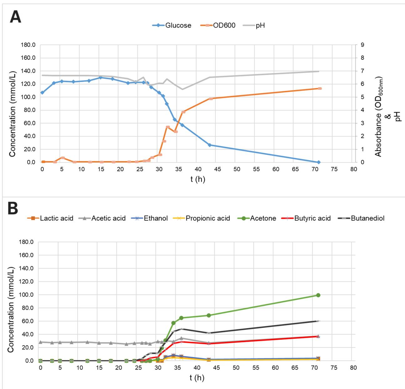
**Fig.12** HPLC results of liquid metabolites in batch samples of *C. acetobutylicum* in Clostridium medium under pH-controlled conditions, showing concentrations (mmol/L) over time (h). **A** shows the glucose concentration combined with OD<sub>600</sub> and pH-level of medium. **B** shows VFA concentrations of lactic acid, acetic acid, ethanol, propionic acid, acetone and butyric acid.
