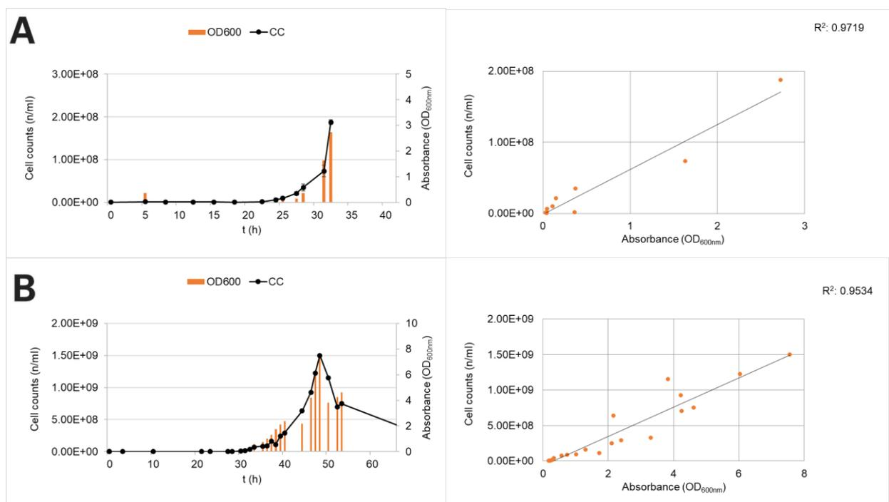
**Fig. 17** Quantification of growth of *C. acetobutylicum* (Clostridium medium) (A) and *E. aerogenes* (Delisa medium) (B) via OD<sub>600</sub> (orange) and cell counts (CC; black line), both under pH-controlled conditions. Additional regression curves analyzing the correlation of OD<sub>600</sub> and cell count-results. Values with high standard deviations were excluded. Standard deviations are shown for the mean values.
