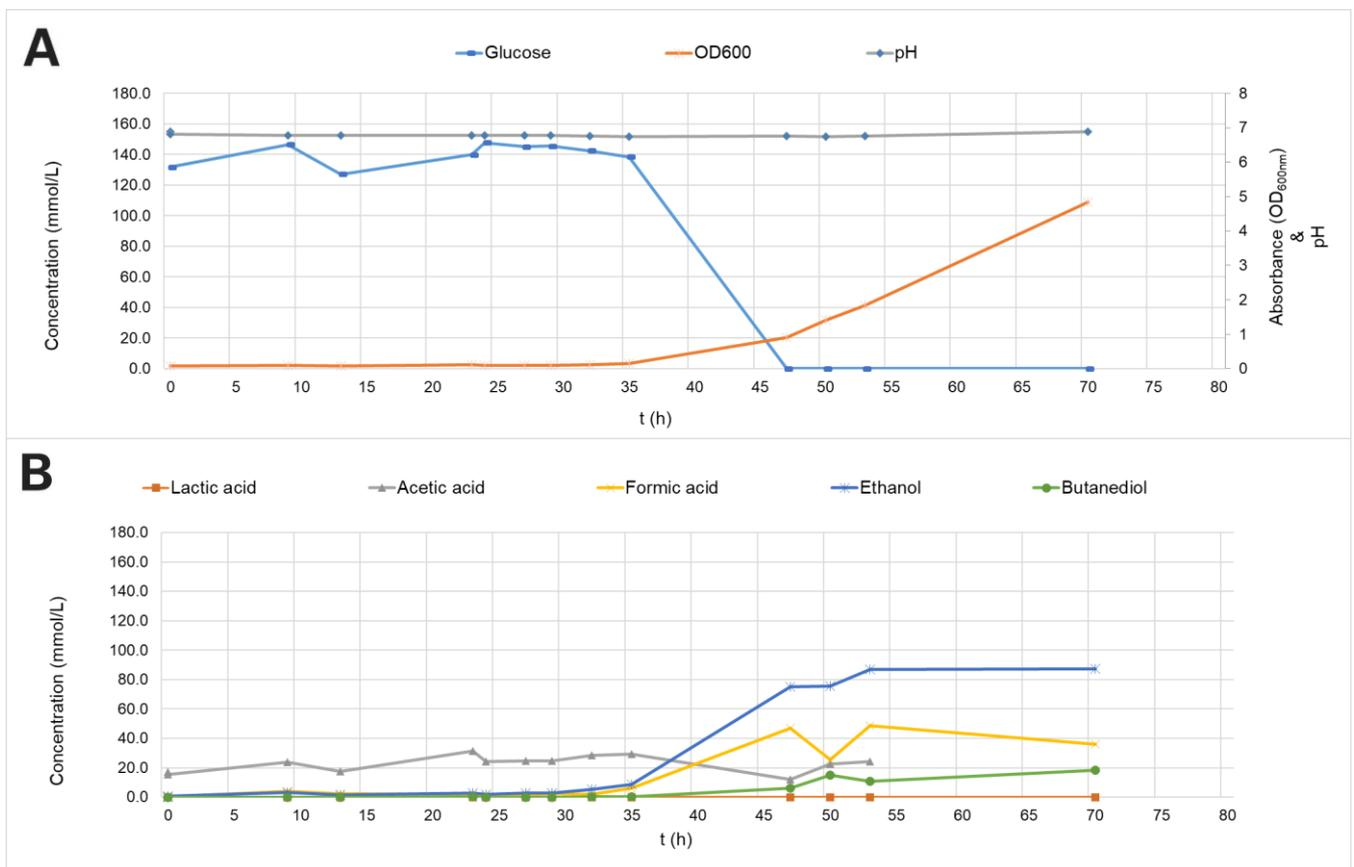
**Fig.13** HPLC results of liquid metabolites in batch samples of co-cultured *C. acetobutylicum* and *E. aerogenes* in DOE E medium under pH-controlled conditions, showing concentrations (mmol/L) over time (h). **A** shows the glucose concentration combined with OD<sub>600</sub> and pH-level of medium over time. **B** shows VFA concentrations of lactic acid, acetic acid, formic acid and ethanol over time. Additionally, concentration of butanediol was measured.
