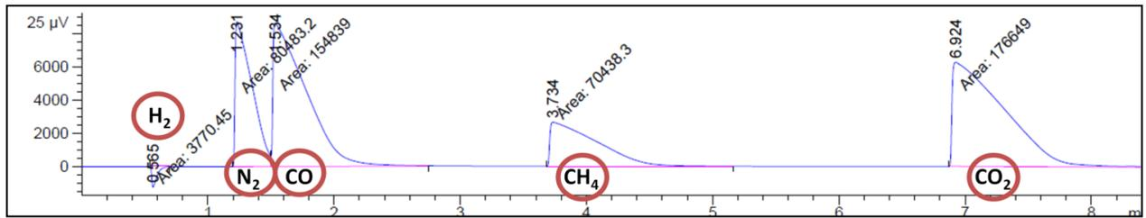
**Fig.1** “Excerpt from gas chromatography analysis. Analysed gases H<sub>2</sub>, N<sub>2</sub>, CO, CH<sub>4</sub> and CO<sub>2</sub> are highlighted” (Reischl, 2016)
