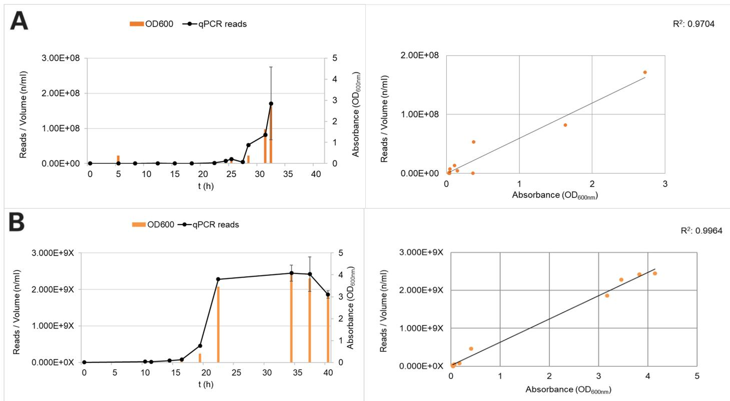
**Fig. 18** Quantification of growth of *C. acetobutylicum* (Clostridium medium) (**A**) and *E. aerogenes* (DOE E medium) (**B**) via OD<sub>600</sub> (orange) and qPCR (black line) under pH-controlled conditions. Additional regression curves analyzing the correlation of OD<sub>600</sub> and qPCR-results (right side). Values with high standard deviations were excluded. Standard deviations are shown for the mean values.
