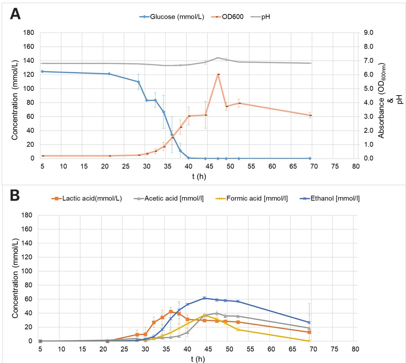
**Fig.9** HPLC results of liquid metabolites in batch samples of *E. aerogenes* in Delisa medium under pH-controlled conditions, showing concentrations over time. **A** shows the glucose concentration combined with OD<sub>600</sub> and pH-level of medium over time. **B** shows VFA concentrations of lactic acid, acetic acid, formic acid and ethanol over time. Standard deviations are shown for the mean values.
