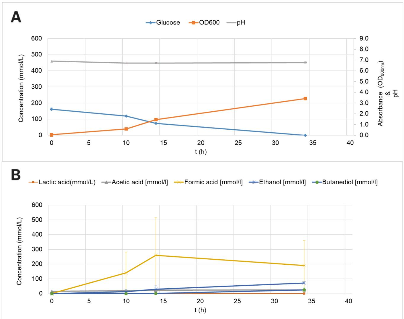
**Fig.10** HPLC results of liquid metabolites in batch samples of *E. aerogenes* in DOE E medium under pH-controlled conditions, showing concentrations over time. **A** shows the glucose concentration combined with OD<sub>600</sub> and pH-level of medium over time. **B** shows VFA concentrations of lactic acid, acetic acid, formic acid and ethanol over time. Additionally, concentration of butanediol was measured. Standard deviations are shown for the mean values.
