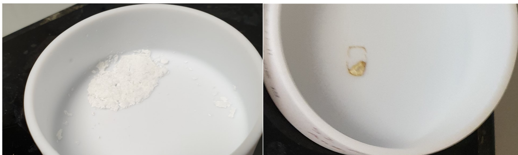
Figure 3.3.3: Dried plutonium fraction after TEVA prior (left) and after (right) the removal of the oxalates from TEVA elution
