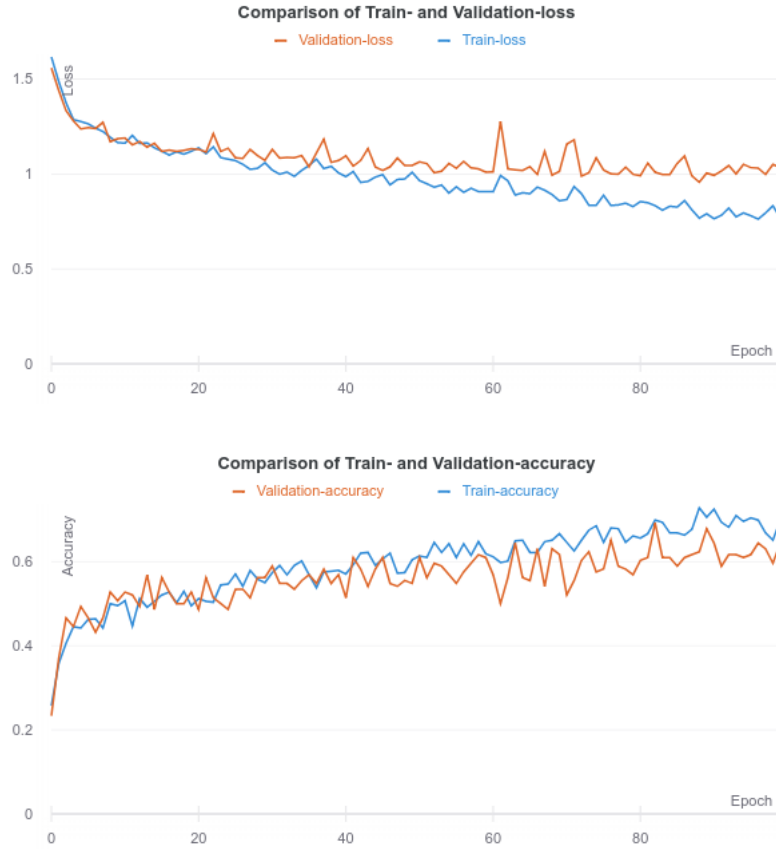
Figure 19: Comparison of loss and accuracy for both the training- and validation-set obtained from using the MLP2 architecture and training for a period of 100 epochs. Above: Loss. Below: Accuracy.
