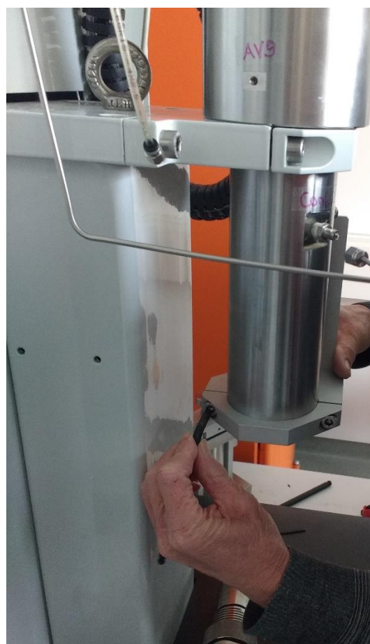
Fig. 8 The Gas-Permeameter-Porosimeter “ Coreval 700 ” at the Department of Geology
