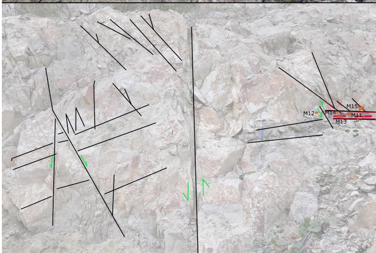
Fig. 29 The conglomerate bed of Outcrop 3 is complexly fractured. The layer described before is situated at the right edge of the picture, where samples are marked with stars.
