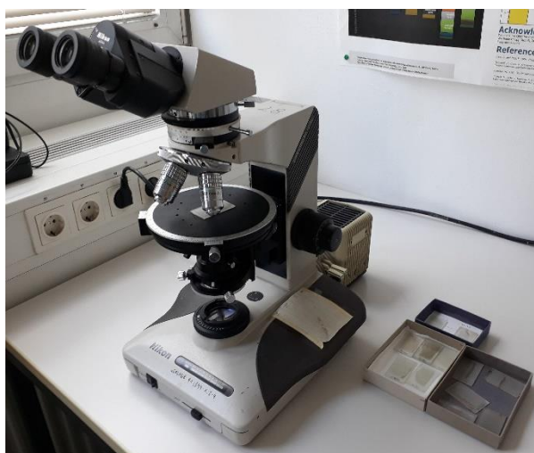
Fig. 5 “Nikon Optiphot 2-Pol” transmitted-light microscope and thin sections of samples M1, M2, M3, M4, M8 and M10
