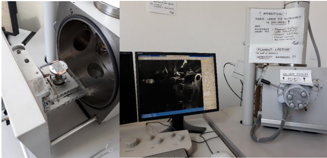
Fig. 6 Photos of the “FEI Inspect S” SEM at the Department of Geology. Left: opened sample chamber with a fixed thin section on the sample table. Right: SEM and monitor.
