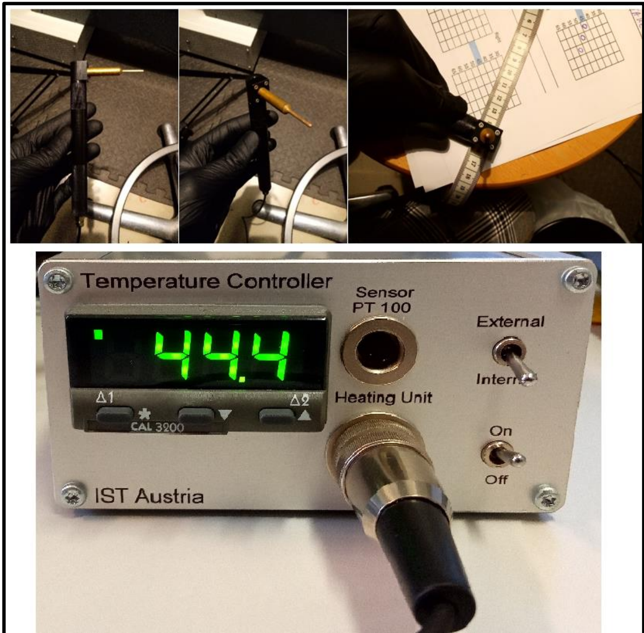
Figure 3. The contact thermode and the temperature controller unit of the punctate heat probe. The upper panel depicts three foreshortenings of the punctate heat probe. The bottom panel depicts the display of the control unit, the temperature adjustment buttons, and the inlet for the PHP. The temperature can be adjusted by using the three buttons underneath the display. Pressing and holding the leftmost button ( \Delta 1 ) enters control mode. The set temperature and the °C symbol start alternating on the screen. The two buttons to the right can then be used to set the required temperature. The left button (arrow down) reduces the temperature and the right increases it. The range used for behavioural experiments was between 30 and 70°C (as reported by the monitor, i.e., actual temperatures of 28.2-62.6°C). Once the required temperature has been set, all buttons can be released. The External/Internal switch should always be kept to the 'Internal' side as this defines that the relative temperature (set on the display) should be measured at the contact thermode and not inside the control box.
