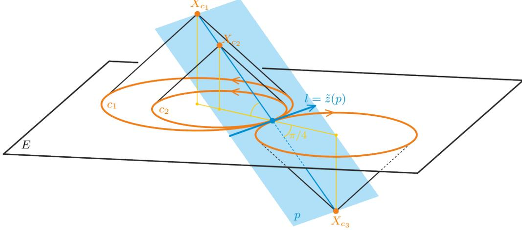
Figure 4.6: Pencil of circles in oriented contact with a common line in  $E$
