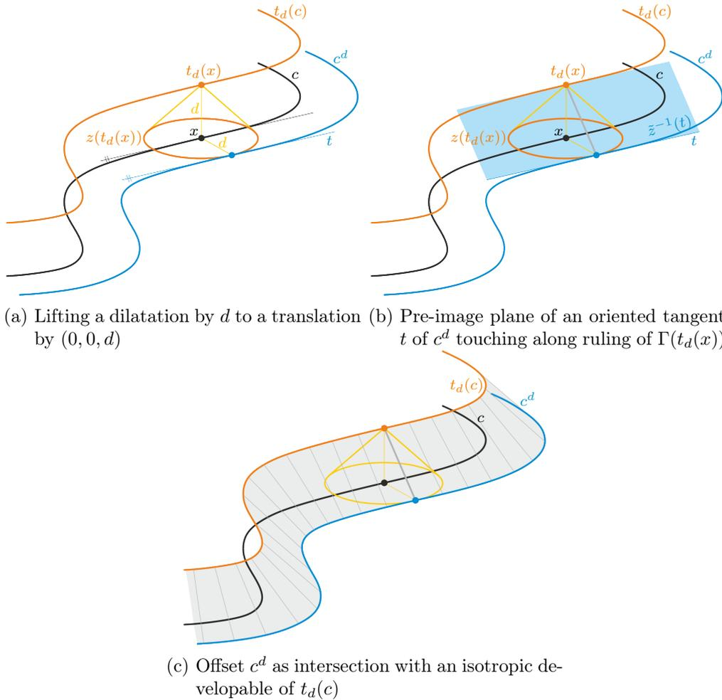
Figure 6.4: Constructing the offset of a planar curve  $c$  within the cyclographic model
