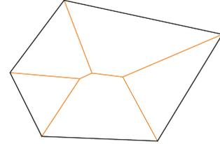
Figure 6.6: Medial axis of a polygon
