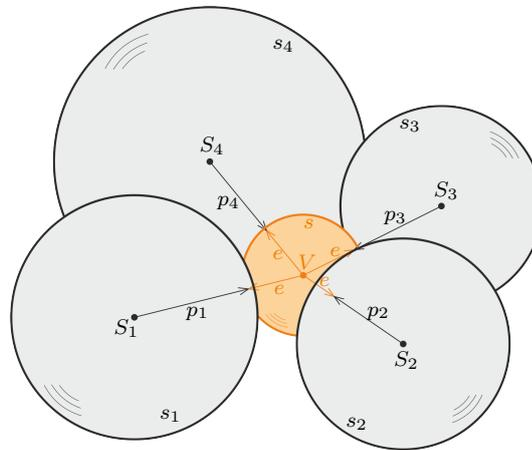
Figure 6.2: The principle of GPS
