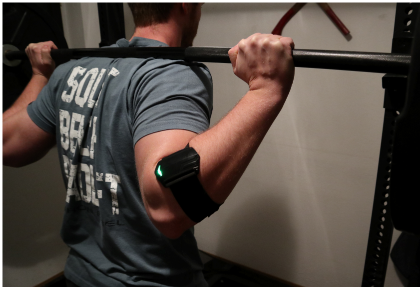
Figure 3.1.: Push Band 2.0 attached at the elbow for the squat exercise. The green light indicates that the exercise has been started in the PUSH application and the device is measuring the mean velocity for the performed repetitions.
