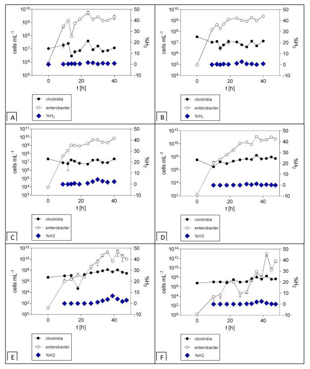
**Figure S1**: Different bioreactor runs with varying initial cell concentrations. A, 1:10; B, 1:100; C, 1:1.000; D, 1:100.000; E, 1:1.000.000; F, 1:10.000.000 for *C. acetobutylicum : E. aerogenes*. Depicted are the respective cell concentrations of *Clostridium acetobutylicum* and *Enterobacter aerogenes*, measured with qPCR, as well as the H<sub>2</sub> concentration in Vol% of the headspace, measured with GC, over the time course of the experiment.
