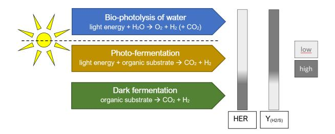
Figure 1: Shown are the three main routes for bio- $H_2$  production plus their respective overall reaction. The sun symbol indicates the light dependency of the two upper processes (Bio-photolysis of water and Photo-fermentation). The dashed line separates the aerobic process (Bio-photolysis of water) from the anaerobic processes (Photo-fermentation and Dark fermentation). Two main features, HER and  $Y_{(H2/S)}$ , are indicated.
