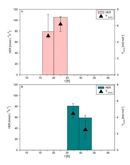
**Figure 1.** HER and  $Y_{(H2/S)}$  results over time for the two best bioreactor runs. The displayed results were achieved when the pH was kept stable at 6, in the top chart, and when the pH was not controlled, in the lower chart. Bars indicate HER; single data plots represent the  $Y_{(H2/S)}$ ; standard deviations are given as error bars.
