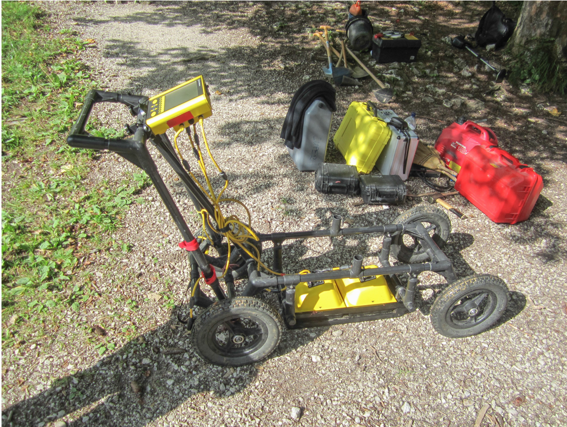
Fig. 4.1: A 500 MHz Tx-Rx antenna from PulseEKKO® PRO system of Sensors & Software mounted on a SmartCart.
