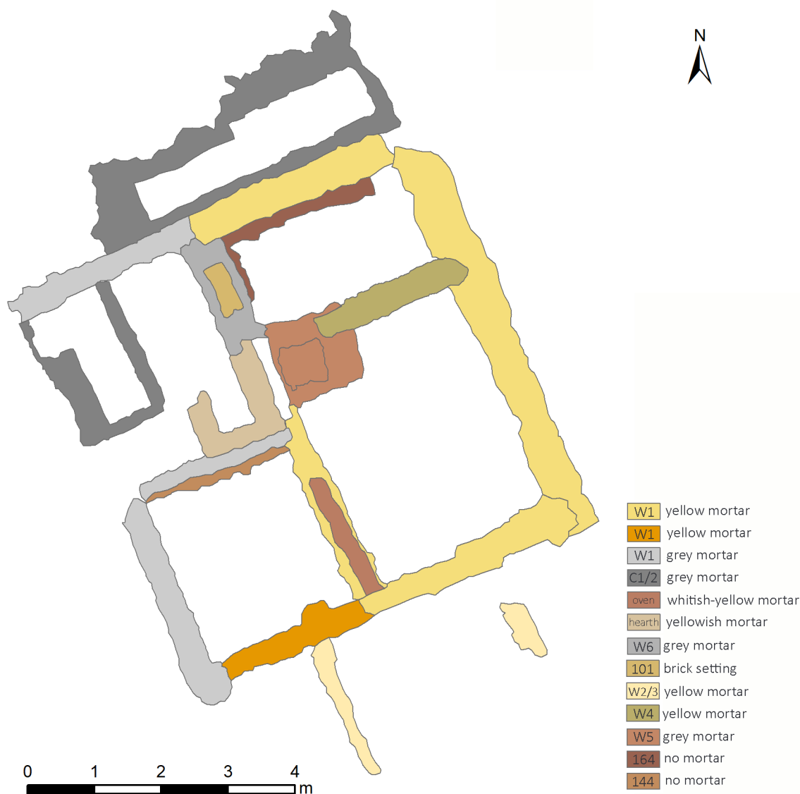
Fig. 7.5: Different mortar types (visually assessed) evidencing different construction phases.
