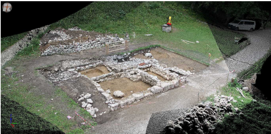
Fig. 4.24: Colored point clouds were gathered with the LMS-Z420i.
