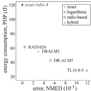
**Fig. 1:** Characteristics of the fixed-point multipliers used in the approximate tensor cores.
