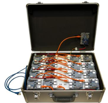
**Fig. 1:** The fully assembled Cluster Coffe. The blue Ethernet cable on the left connects to the outside world.
