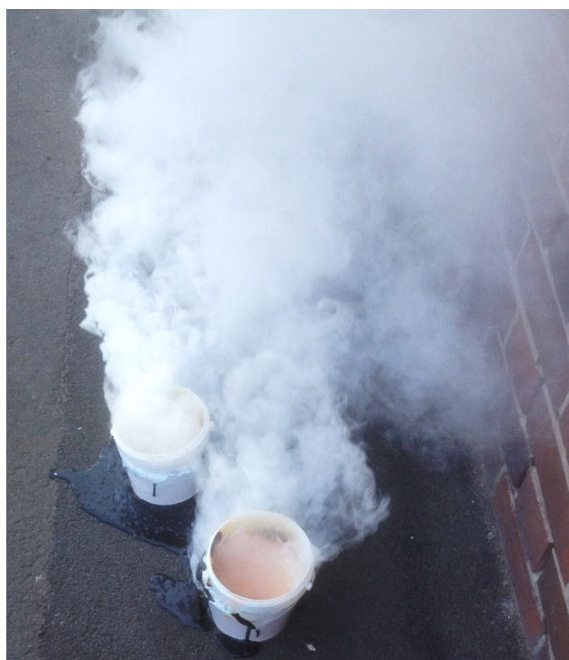
Figure S1: A photograph of buckets containing a mechanically frothed epoxy formulation Epoxy L (EPL) and hardener GL1, purchased from R&G Faserverbundwerkstoffe GmbH (Waldenbuch, Germany) formulation, which started curing during frothing in an industrial mixer (Henschel). We had to discharge the curing formulation quickly from the mixer and distinguish the fire. The material remaining in the mixer we had to remove mechanically – a time consuming undertaking. The highly exothermic curing reaction of epoxy resins can easily result in charring of the resin and even fire of the material, if the heat cannot be dissipated properly, which is difficult if the material contains in excess of 70 vol.% dispersed air.
