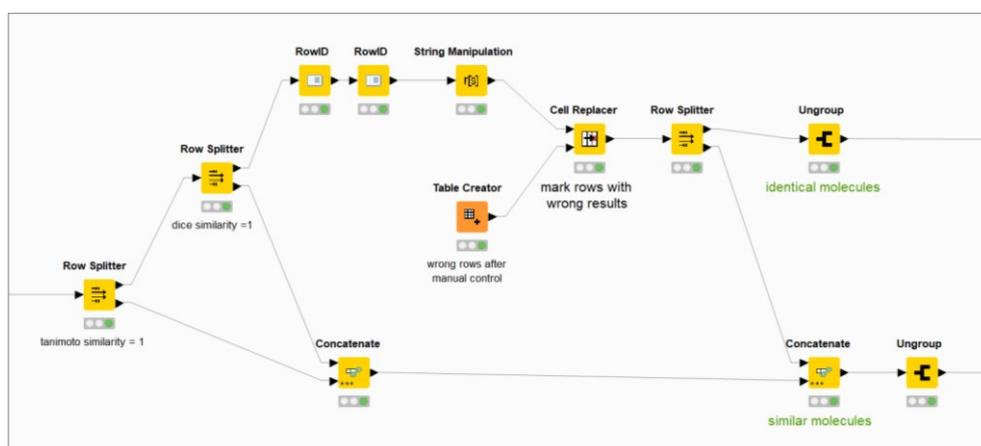
FIGURE 17: Separating rows with identical molecule matches from rows with non-identical matches
