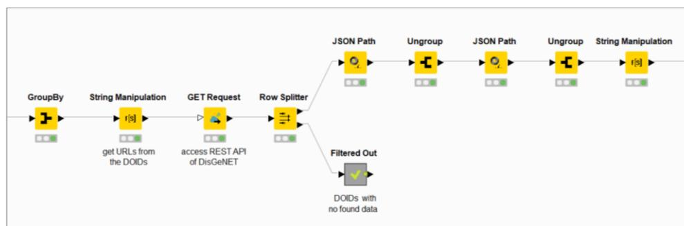
FIGURE 6: Accessing DisGeNET through its REST API and transforming the JSON formatted data into separated readable columns
