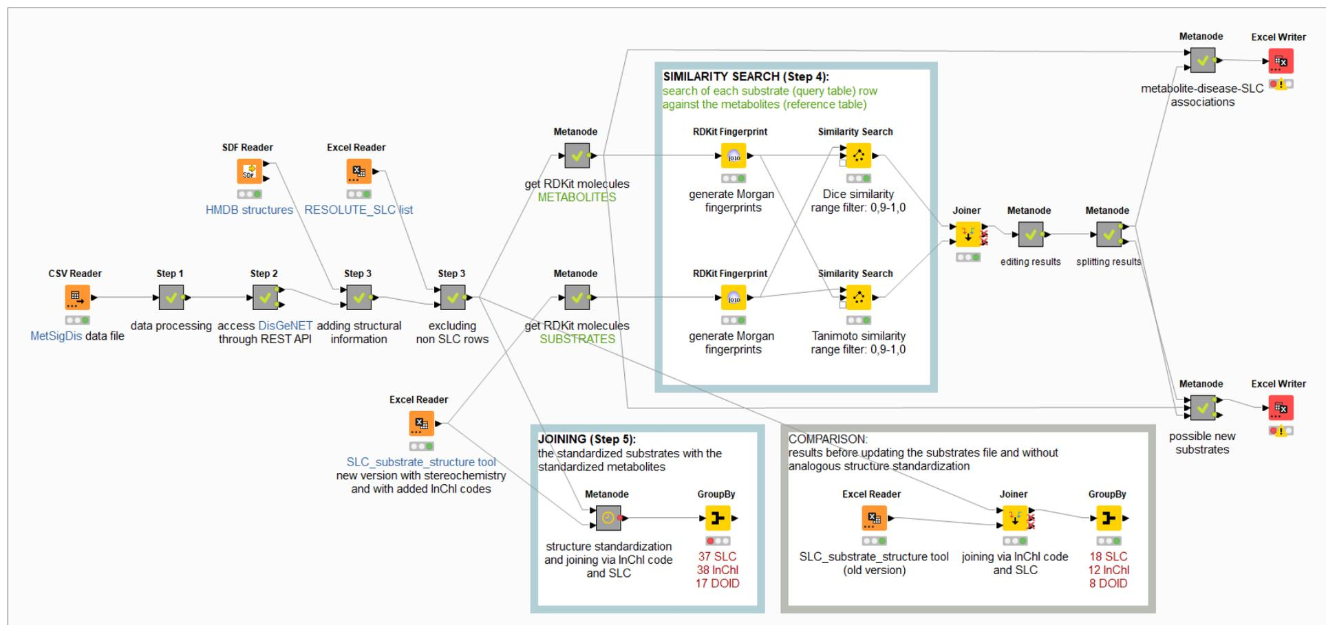
FIGURE 26: Workflow for the connection of disease associated alterations of metabolites with corresponding SLC transporters
