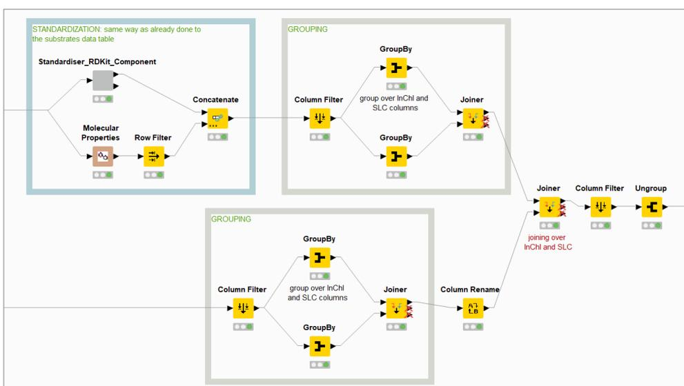
FIGURE 21: Overview of the joining approach: First the structure standardisation of the metabolite structures, then the same grouping step for both the metabolites table and the substrates table, followed by the joining via InChI codes and SLCs.
