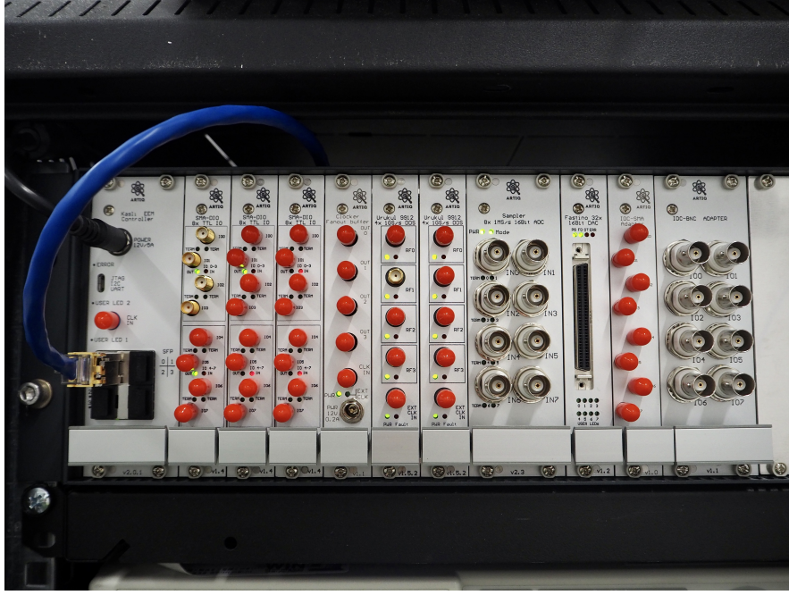
Figure 3.2: Frontpanel of the Sinara and its Modules: From left to right: Kasli FPGA-carrier, 3x DIO-SMA, Clocer, 2x Urukul, Sampler ADC, Fastino DAC, and its corresponding IDC-SMA and IDC-BNC adapter.
