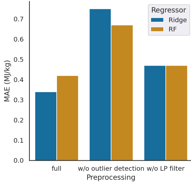
Figure 3.11: On the fully preprocessed data, ridge regression outperforms RF regressors. However, that is not the case for data that has not been carefully preprocessed. (RFs with twenty limited trees, ridge regression with a regularisation \alpha of 1.0 and the one year training set.)
