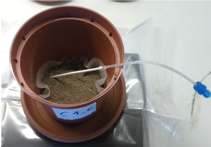
Figure 6: Rhizon sampler for pore water samplings in one of the pots for the experiment, own photography.
