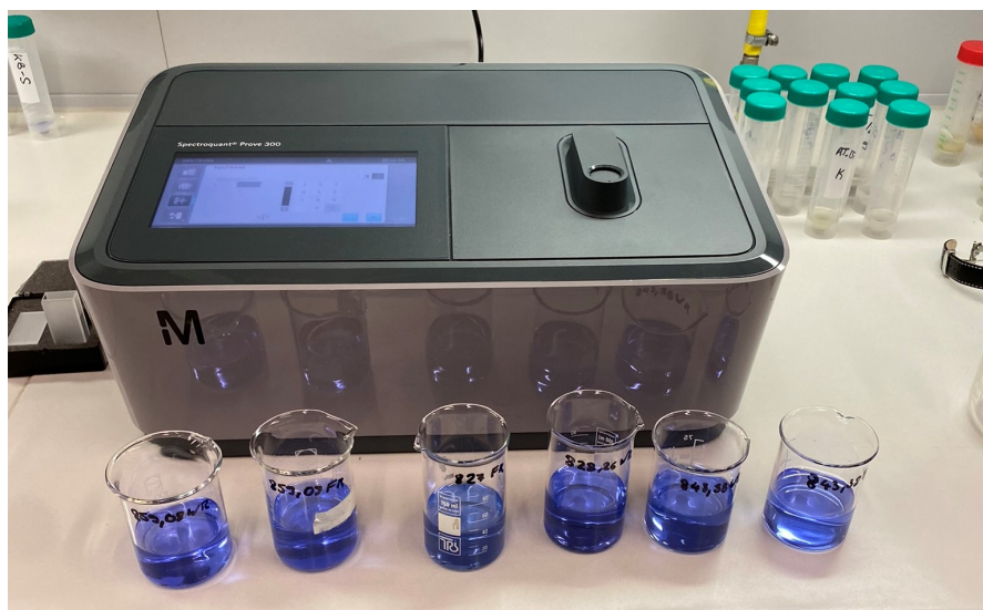
Figure 2.6: Spectrophotometer with Cu-complex solution of samples. Differences in ion concentration are measured with the Spectrophotometer.
