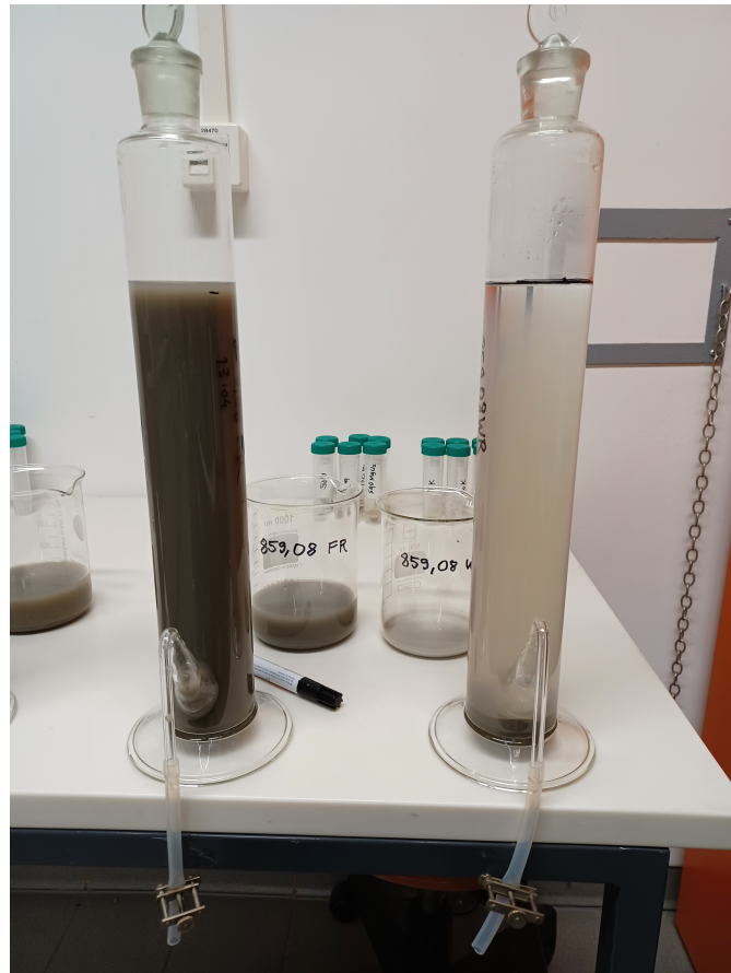
Figure A.4: left: Atterberg-cylinder with clay particles in suspension (stable clay suspension). right: Atterberg-cylinder with flocculated/aggregated clay particles on the bottom (unstable clay suspension).
