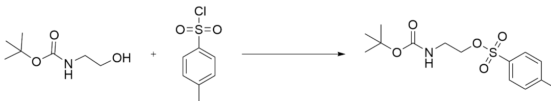
Figure 30: Reaction scheme for the synthesis of 2-(tert-butoxycarbonylamino)ethyl-4-methylbenzenesulfonate
