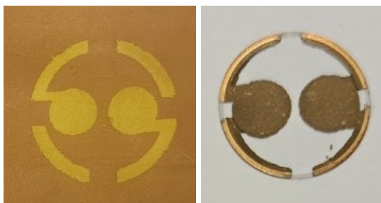
Figure 19: QCM gold electrodes applied by screen-printing. Left: Stencil used for applying the gold paste. Right: The resulting electrodes.
