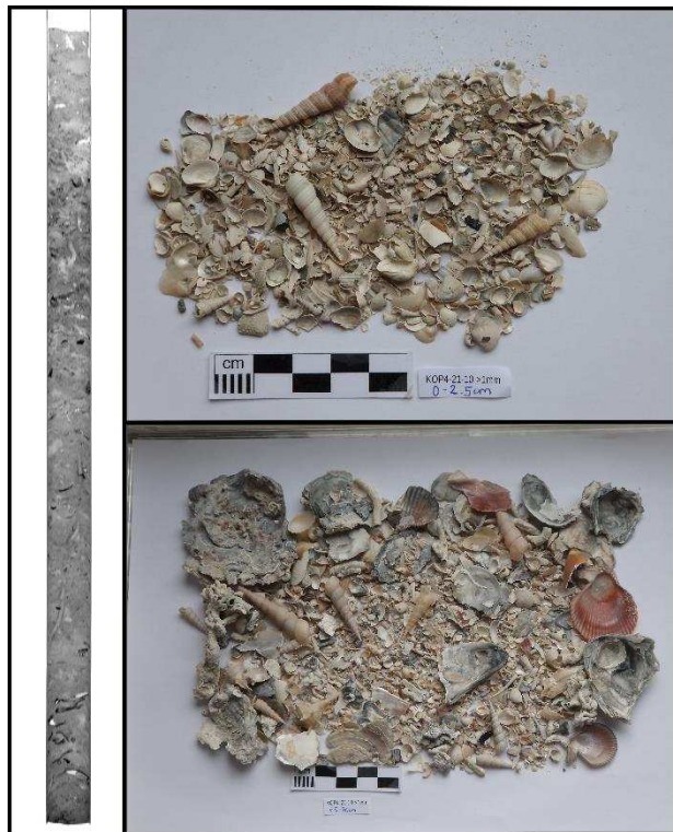
Figure 2. Left: Radiographic image of core KOP4-21-9. The lighter the grey shading, the higher the sediment density. Right: >1-mm sieve fraction of two increments (0-2.5 and 65-70 cm) from core KOP4-21-10. Note the prevalence of shells and biogenic debris.
